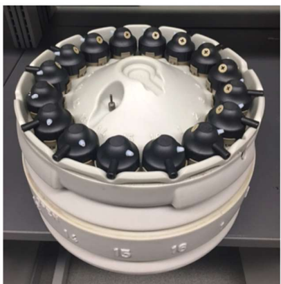
Figure 11: Two rotors and their accompanying vessels, 24HVT50 and 16HF100, were often used for the microwave acid digestion of both algal and HTL solids. The rotor and vessels 16HF100 were determined to be the ideal for complete digestion for both algal and HTL solids.
