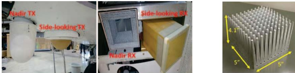
Figure 2.2: Transmit and Receive antennas mounted on front and back of the Twin Otter aircraft (left & middle) and Vivaldi array antenna (right) for off-nadir mode [24]
