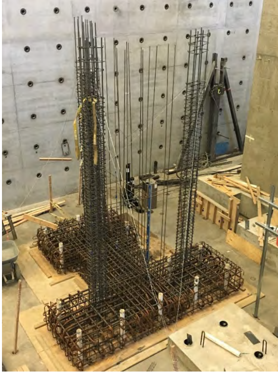
(a) Base block steel cage
