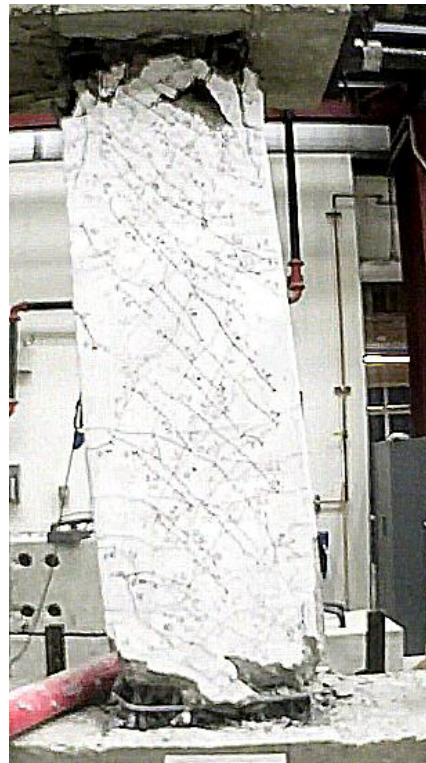
Figure C.65 – D100-3.5 at -8% chord rotation, second cycle
