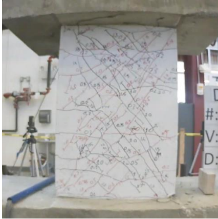
Figure C.16 – D120-1.5 at +2% chord rotation, second cycle
