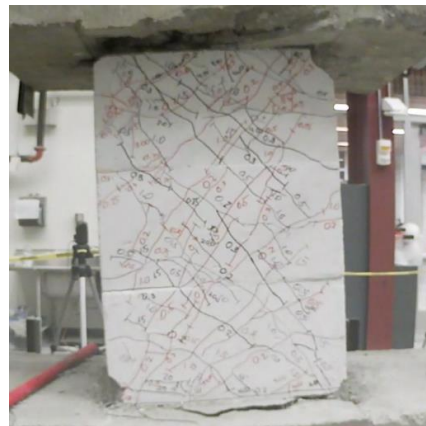
Figure C.12 – D100-1.5 at -4% chord rotation, second cycle
