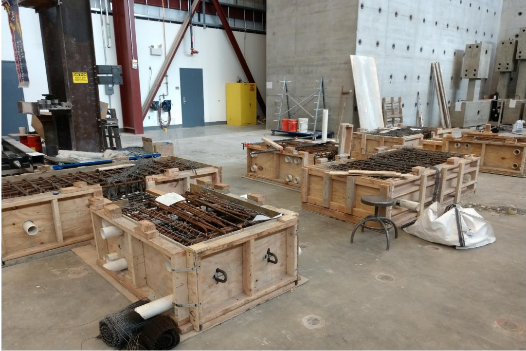
Figure B.5 – Specimens prior to casting, D80-1.5, D100-1.5, and D120-1.5 (from left to right)
