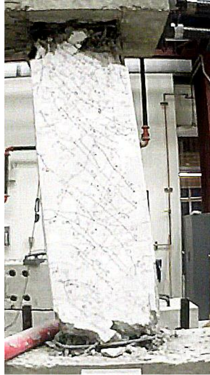
Figure C.67 – D100-3.5 at -10% chord rotation, first cycle
