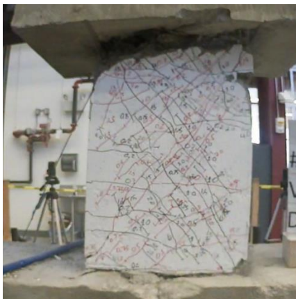
Figure C.18 – D120-1.5 at +4% chord rotation, second cycle
