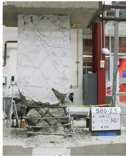
Figure C.81 – P80-2.5 at -6% chord rotation, second cycle
