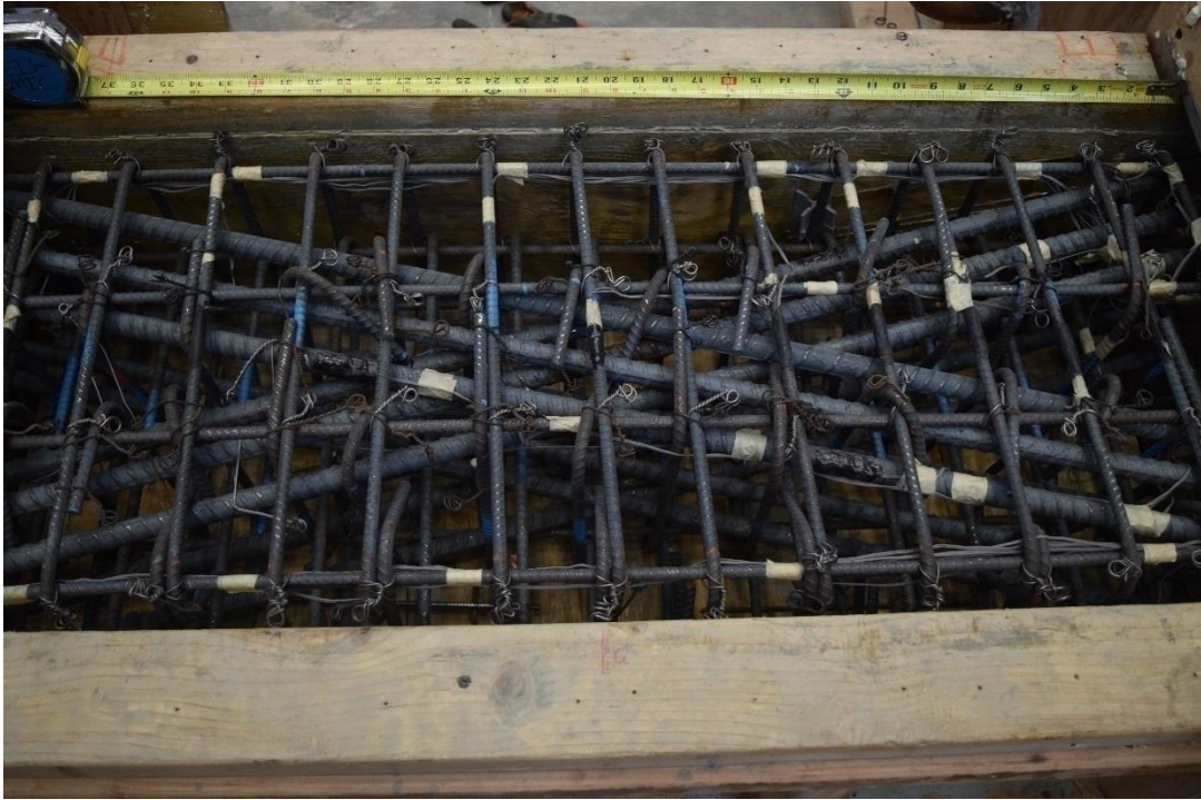
Figure B.1 – Coupling beam reinforcement, D120-2.5
