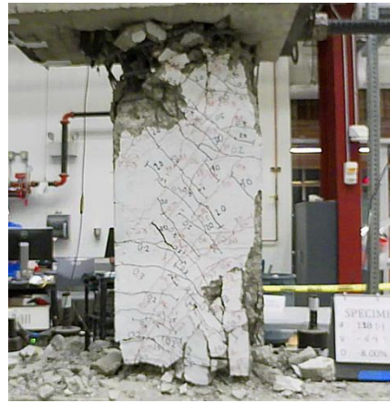
Figure C.31 – D80-2.5 at -10% chord rotation, first cycle
