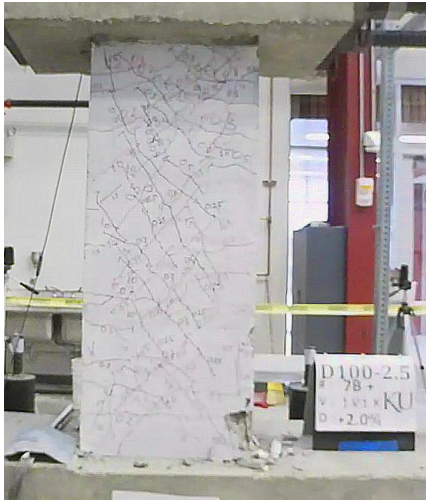
Figure C.32 – D100-2.5 at +2% chord rotation, second cycle
