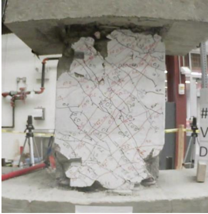
Figure C.5 – D80-1.5 at +6% chord rotation, second cycle
