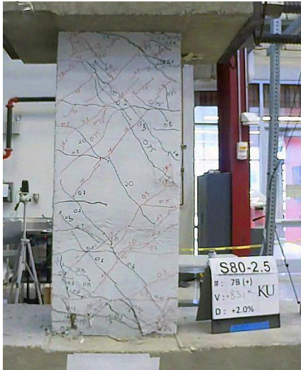
Figure C.76 – P80-2.5 at +2% chord rotation, second cycle
