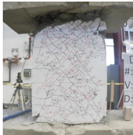
Figure C.19 – D120-1.5 at -4% chord rotation, second cycle
