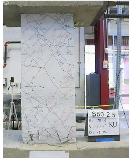
Figure C.77 – P80-2.5 at -2% chord rotation, second cycle
