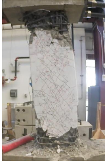
Figure C.57 – D80-3.5 at -10% chord rotation, first cycle
