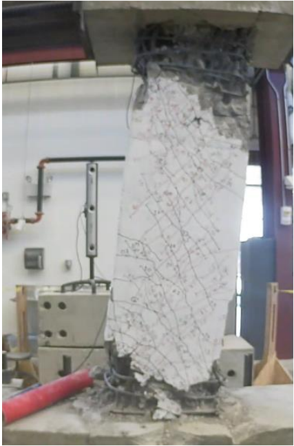
Figure C.56 – D80-3.5 at +10% chord rotation, first cycle
