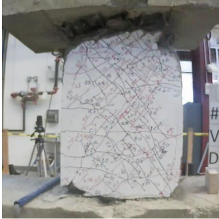
Figure C.20 – D120-1.5 at +6% chord rotation, first cycle
