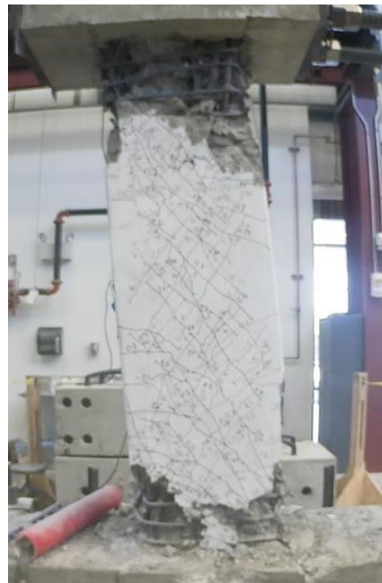
Figure C.55 – D80-3.5 at -8% chord rotation, second cycle
