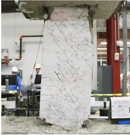
Figure C.26 – D80-2.5 at +6% chord rotation, second cycle
