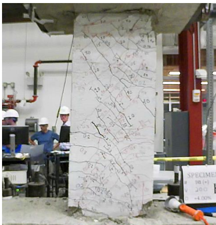
Figure C.24 – D80-2.5 at +4% chord rotation, second cycle
