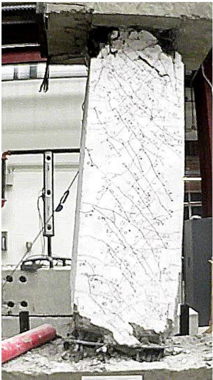
Figure C.64 – D100-3.5 at +8% chord rotation, second cycle
