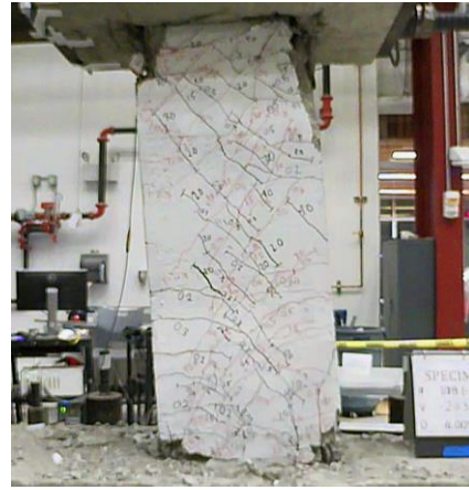
Figure C.27 – D80-2.5 at -6% chord rotation, second cycle
