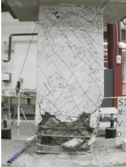
Figure C.86 – P100-2.5 at +6% chord rotation, second cycle
