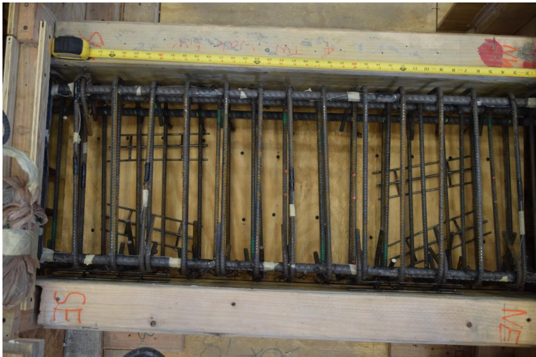
Figure B.2 – Coupling beam reinforcement, P100-2.5
