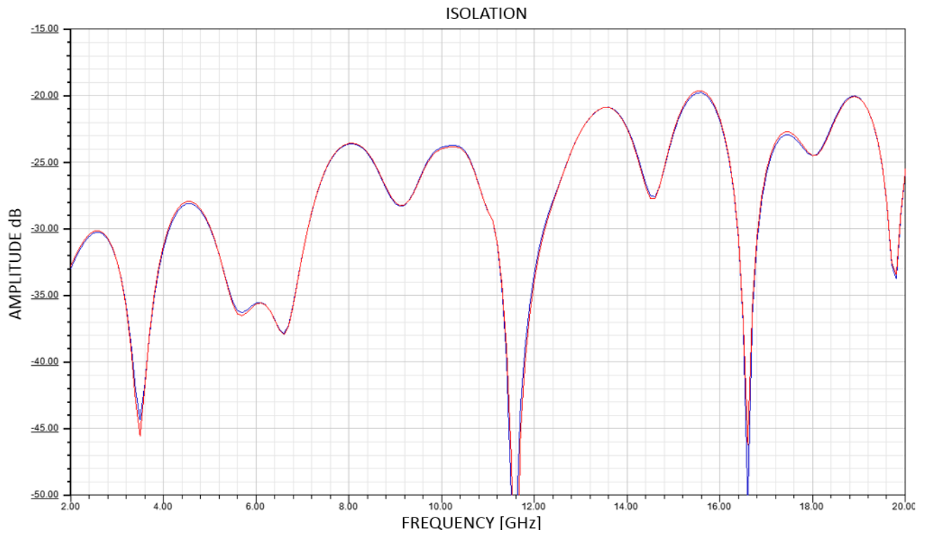
Figure 4.1.5: HFSS simulation of the isolation between the wave ports and corresponding isolation wave ports
