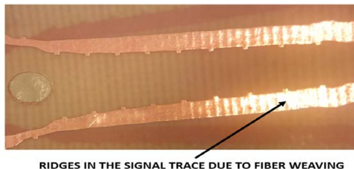
Figure 4.6.3.1: Ridges on the copper trace caused due to reinforcement fiber weaves in the dielectric laminate material
