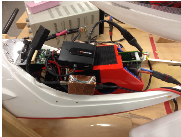
Figure B.4: Picture of our avionics containing a usb hub
