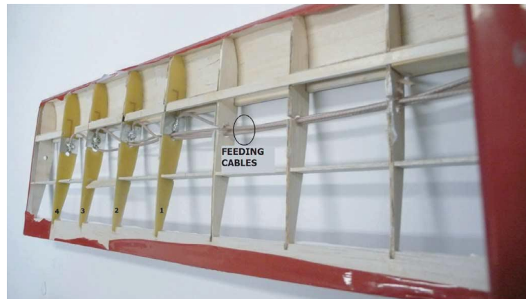
Figure 8: Printed antenna array into wing structure [16]
