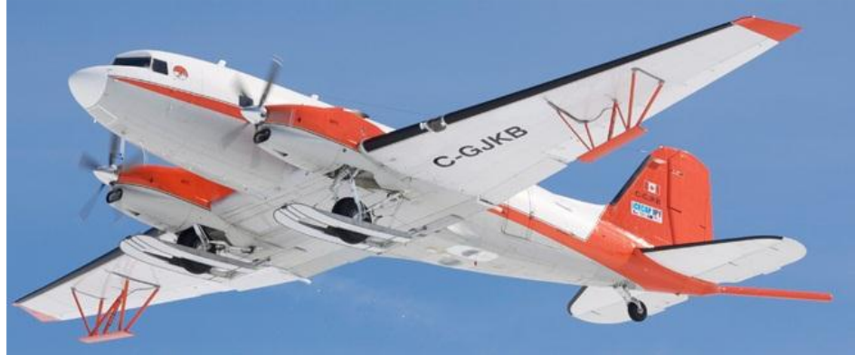
Figure 9: HiCARS installed on Basler (Photo courtesy of UTIG) [12]
