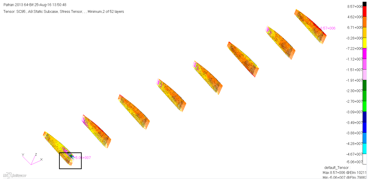
Figure 123: Rib maximum transverse compression stress plot
