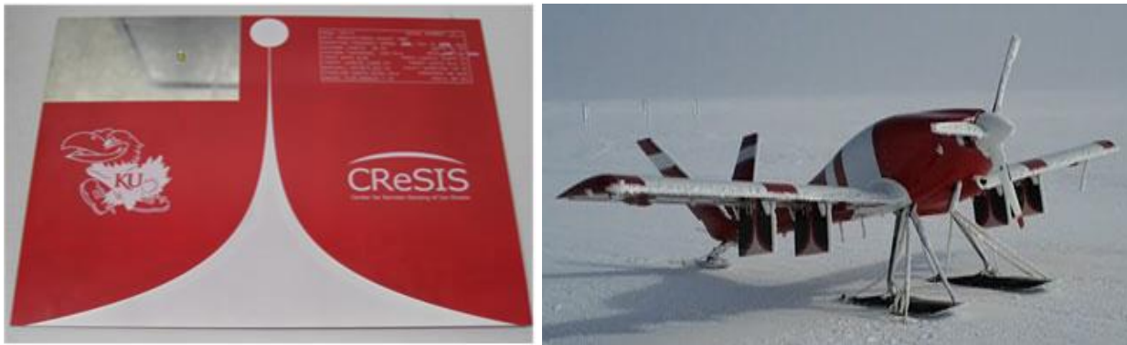
Figure 1: Vivaldi Antenna [8] (left) and Meridian UAS with four antennas integrated below wing [9] (right)
