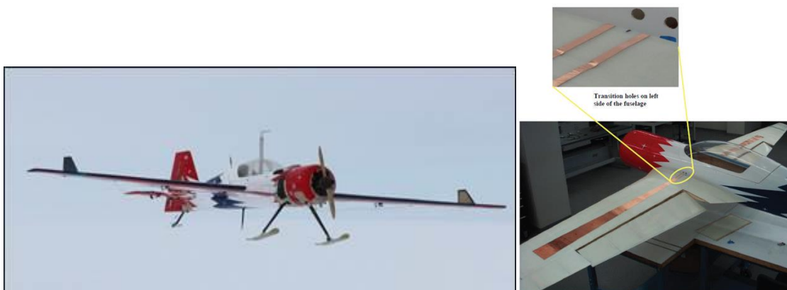
Figure 7: The G1X UAS in flight (left) (Credit: Dr. Shawn Keshmiri, KUAE) and antennas integrated on the wing (right) [15]
