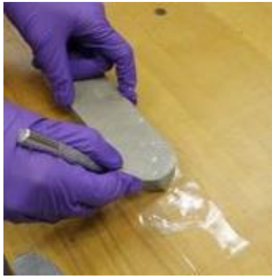
Figure 20: Covering the surface of cores with transparent tape (Picture taken by Reza Barati-used with permission)
