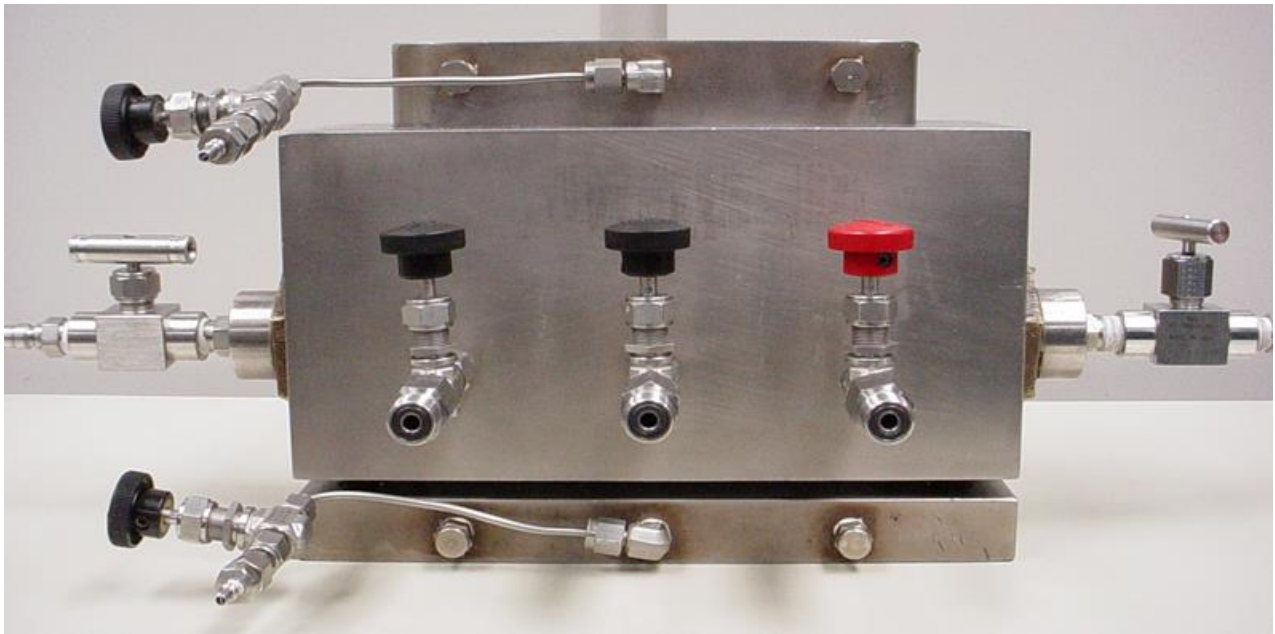
Figure 18: Picture of the fracture conductivity cell provided by Schlumberger
