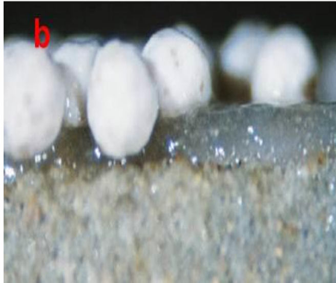
Figure 2: Filter cake reducing fracture width [33] Stimlab
