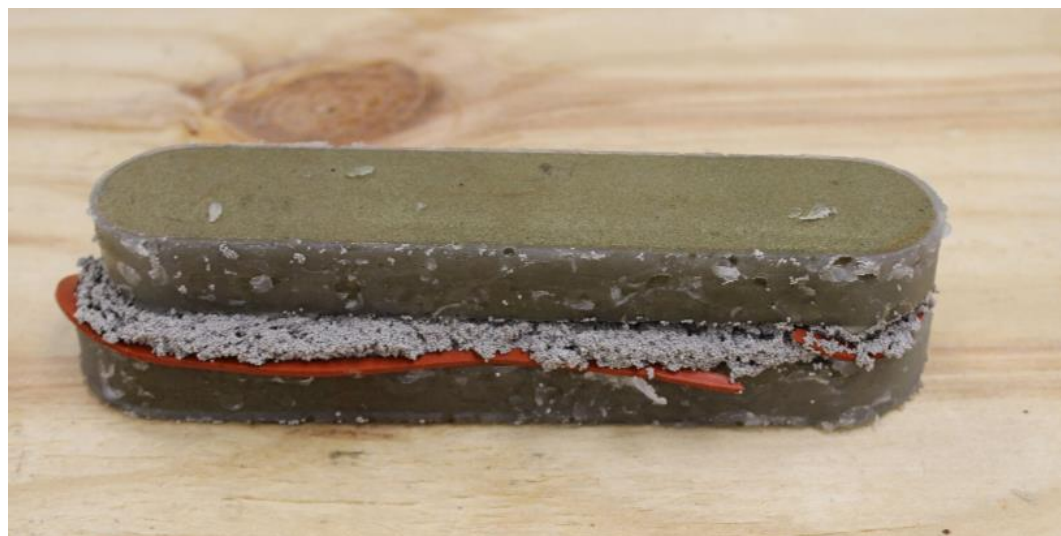
Figure 32: Cores with the proppant pack after the conductivity test
