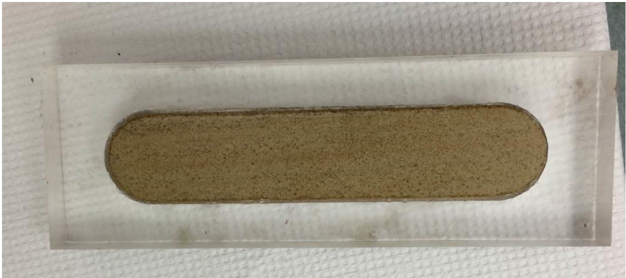
Figure 22: Sealed and dried Core inside the core holder
