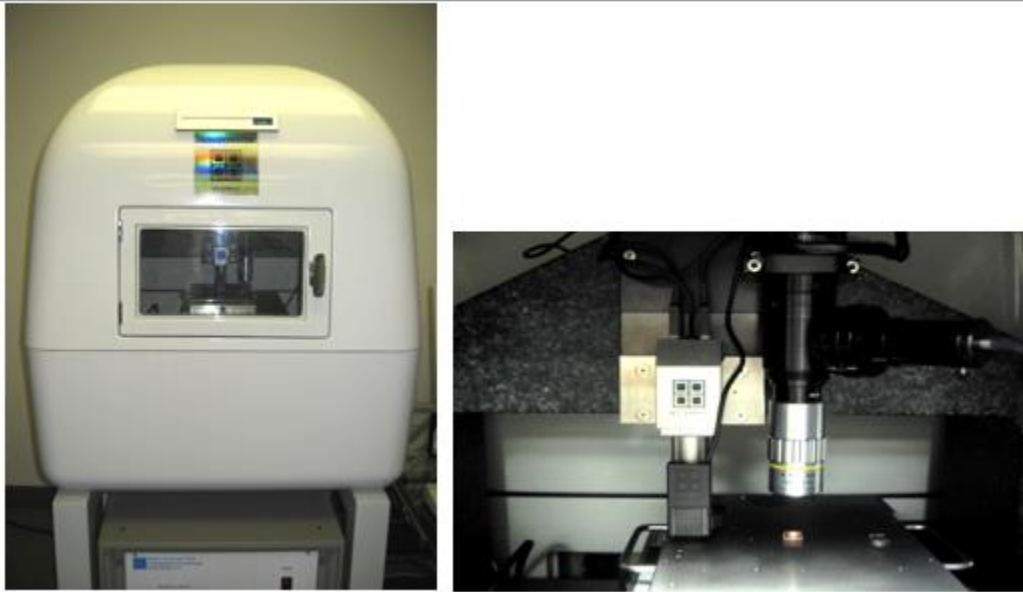
Figure 12: The full-feature, multi-technique nano-mechanical test system; Left: main unit; Right: transducers mounted on a granite platform inside the environmental enclosure [77]
