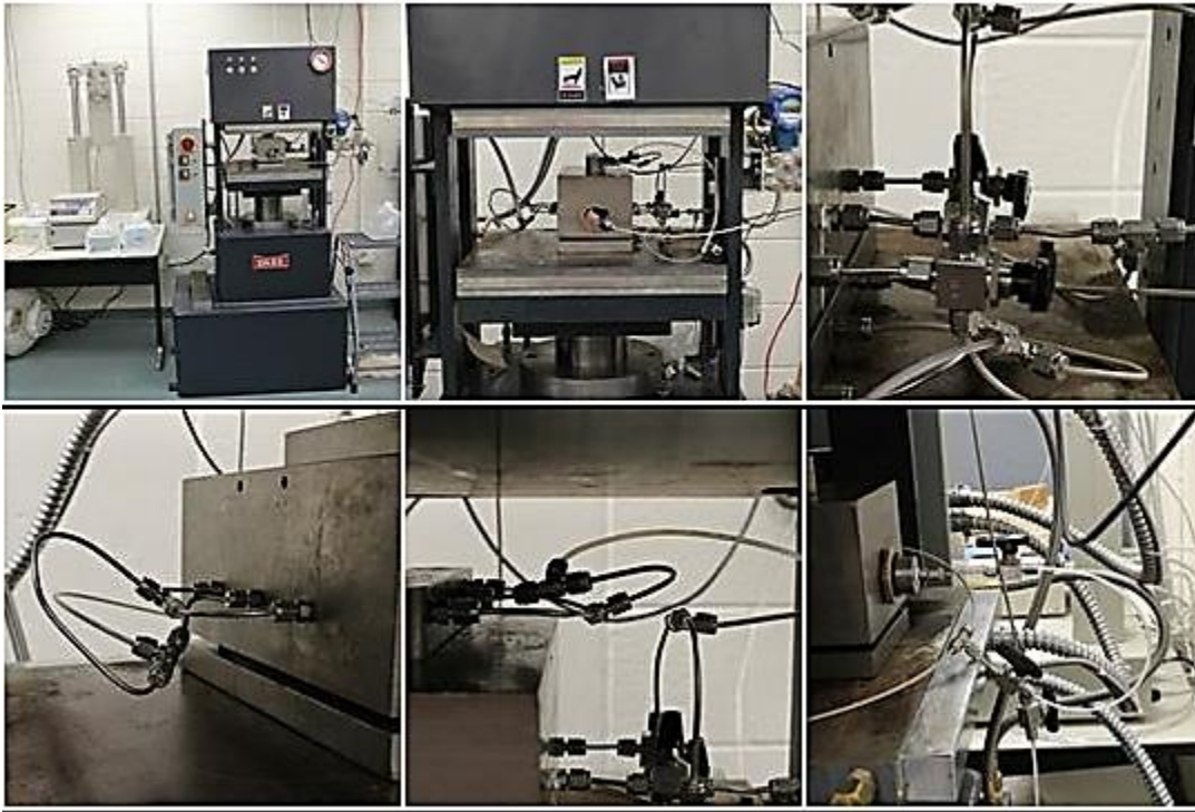
Figure 31: Fracture conductivity cell with the flow lines during the test
