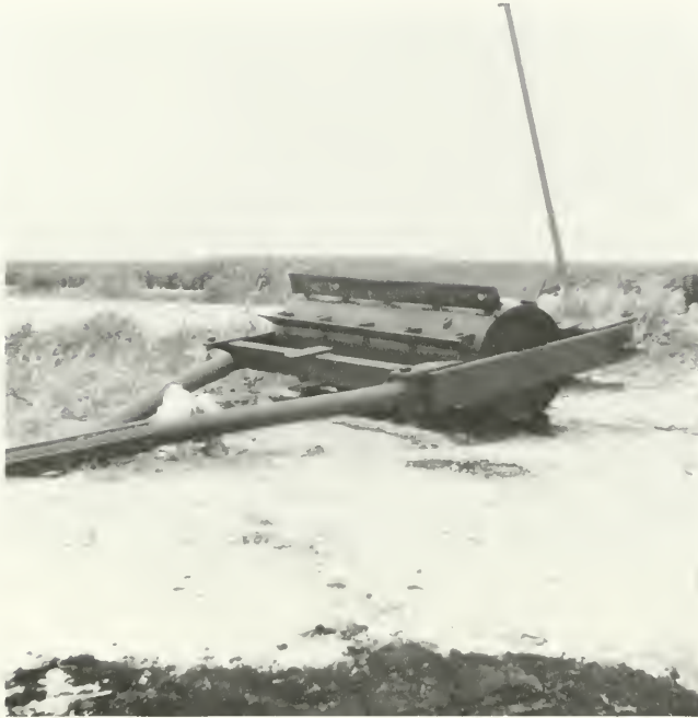
FIGURE 34. The "devil catcher," used to control plant growth along canal banks in western Broward and Palm Beach counties, leaves a path of destruction in its wake. (JR)
