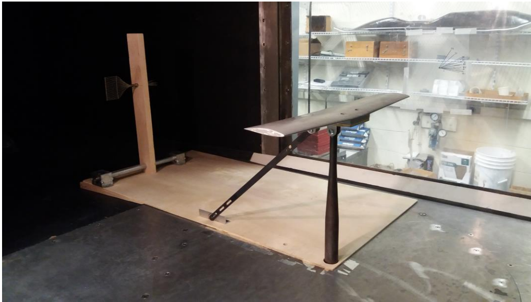
Figure 5.9: CAD vs Test Board with Wing Model Attached
