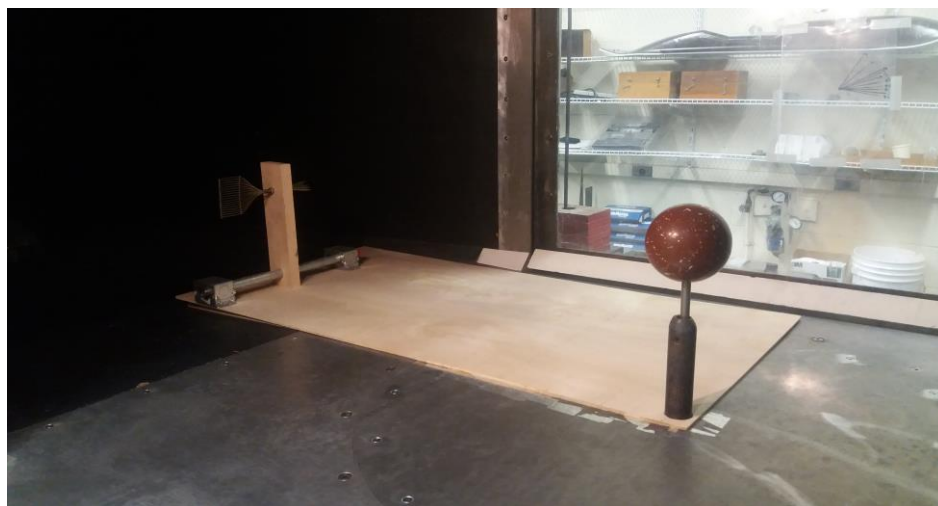
Figure 5.6: CAD v Test Board with Sphere Model Attached
