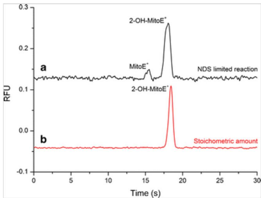
**Fig. 2.** MitoHE reaction with NDS prepared using (a) 3.6 mg of potassium NDS (NDS limited reaction) and (b) using 4.0 mg of potassium NDS (stoichiometric amount) from a 67.5 % pure Fremy's salt. Laser alignment at 2.3 cm
