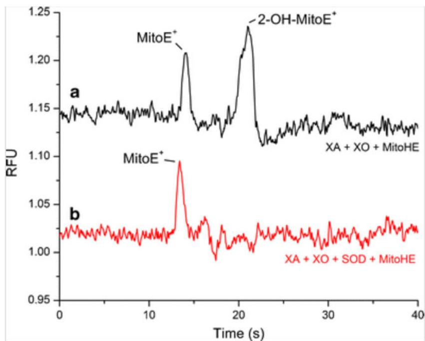
**Fig. 3.** Electropherograms for the injection of XA/XO reaction media + MitoHE with and without SOD
