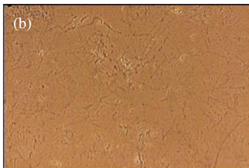
Figure 3.3. (a) Photo of silicon wafer after 1 minute exposure to copper plating solution with 0.27 M \text{NH}_4\text{F} and 0.13 M \text{Cu}^{2+} . (b) Optical image of same wafer from part (a).
