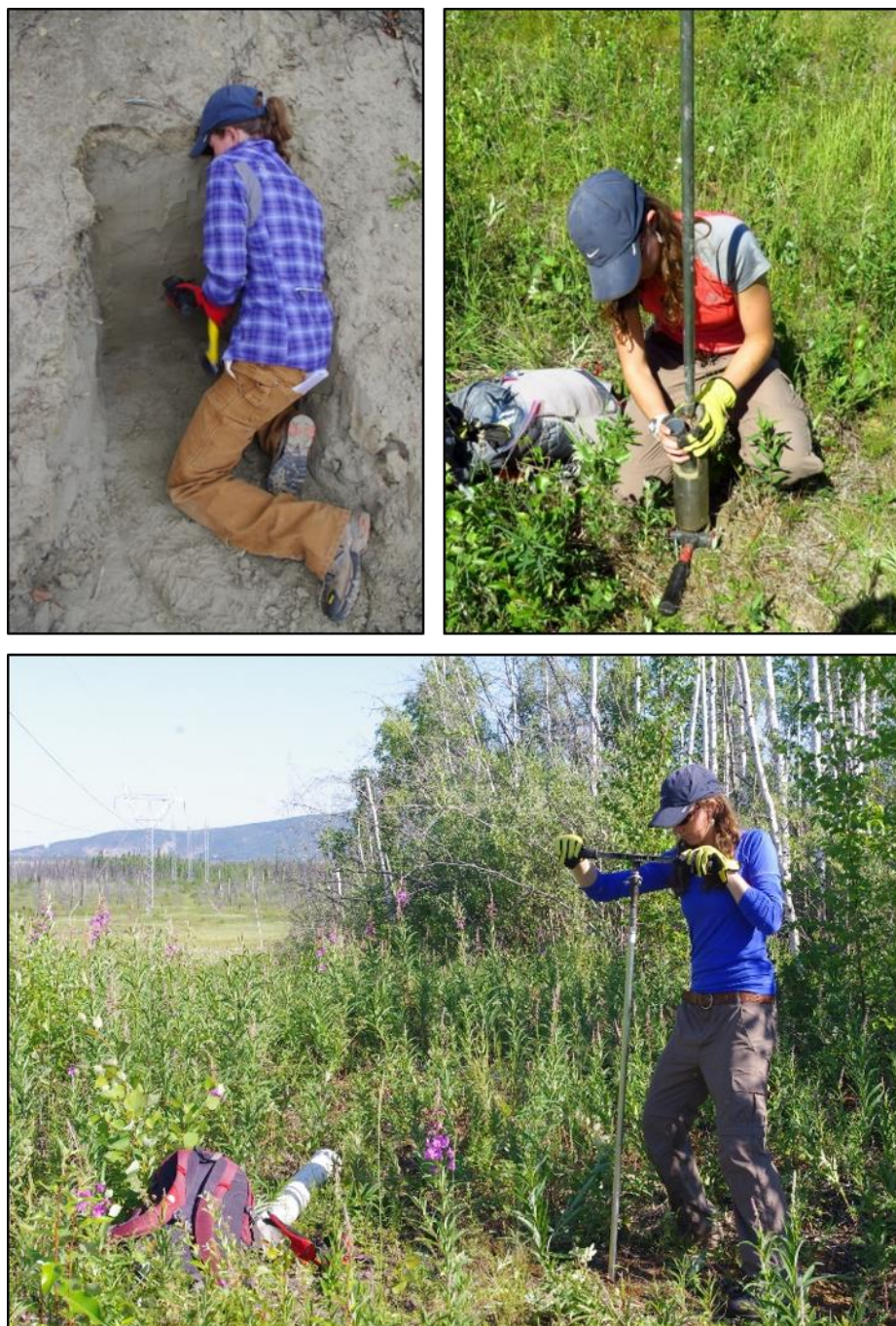
Figure 4.3. Various sampling techniques used in the field. Top left: At road cut sites where establishment of stratigraphic profiles was possible, tubes were hammered in to the sediment and then sealed with black vinyl end caps. Bottom: Bucket auguring was employed to collect luminescence samples at sites without natural exposures. Top right: The tubes were then inserted into the auger bucket to capture the sediment (Photographs: W. Johnson and C. Messner).
