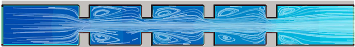
Figure 4-3. Representative Plan View from HEC-RAS 2D Showing Typical Flow Patterns from the Simulations.
