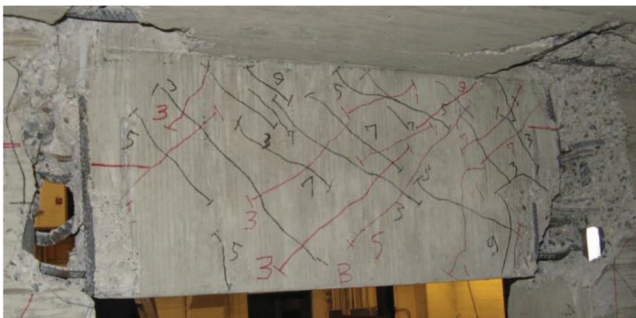
(a) Specimen CW-1: Typical beam damage (2 nd floor beam pictured)
