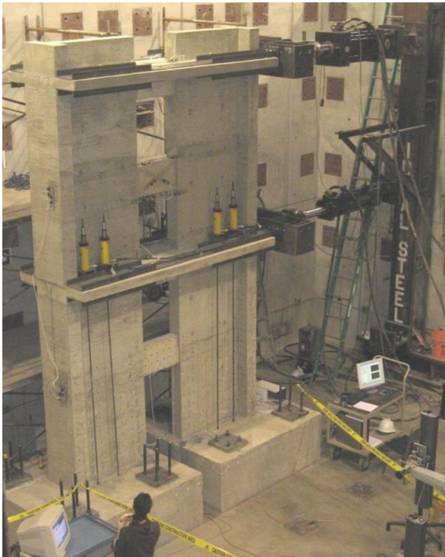
Fig. 1—Coupled wall specimen, before testing.
