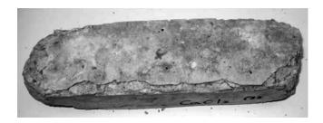
Fig. 9—Specimen subjected to 10 weeks of exposure to 6.04 molal ion concentration solution of CaCl<sub>2</sub>.
