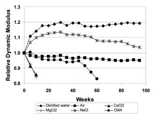
Fig. 1—Relative dynamic modulus of elasticity (wet-dry)  $P_{w/d}$  versus number of weekly wet-dry cycles for specimens exposed to 6.04 molal ion concentration deicer solutions.
