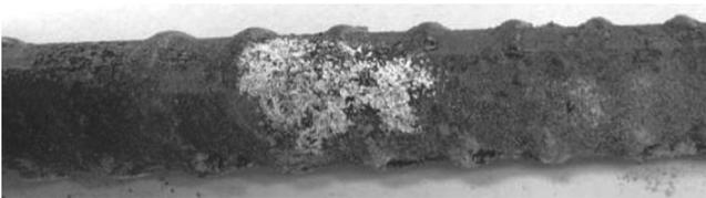
Fig. 6—Bar from Specimen Z-B-8 after autopsy. Corrosion product on top bar. Nominal bar diameter = 5/8 in. (16 mm).
