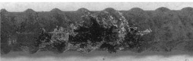
Fig. 7—Bar from Specimen Z-B-3 after autopsy. Corrosion product on top bar showing intermetallic layer. Nominal bar diameter = 5/8 in. (16 mm).
