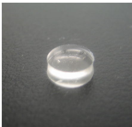
Figure 5.4. Representative image of a HA-DVS disc used to carry out swelling and mechanical testing. The discs were 5 mm in diameter and had a height of 2 mm.
