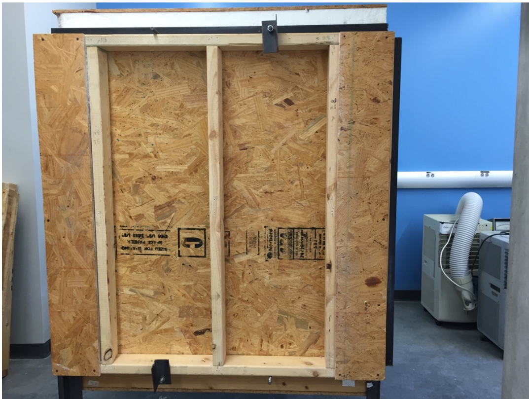
Figure 3.3 Wall Panel Cavity
