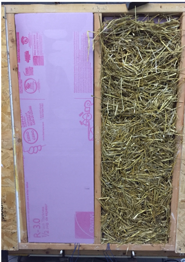
Figure 3.9 Cavity Filled with Straw
