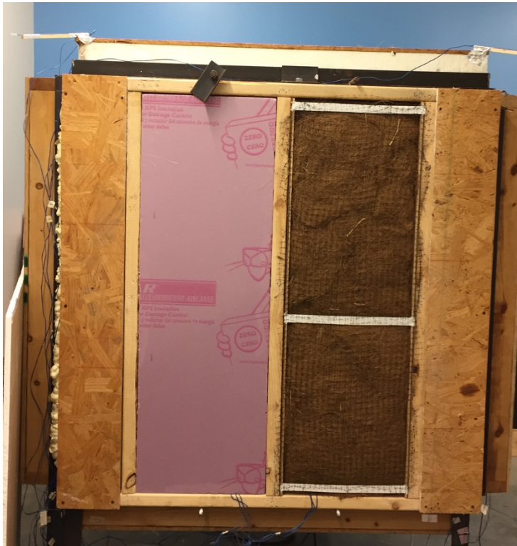
Figure 3.11 Removable Cavity Panel with Coconut Fiber
