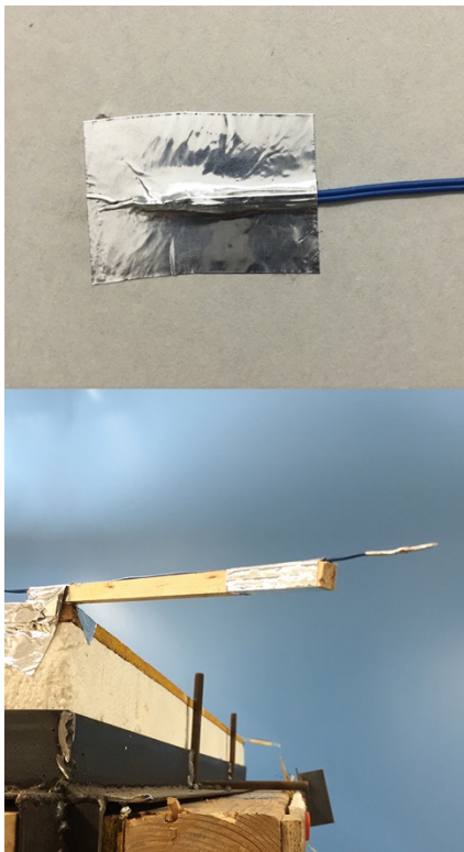
Figure 3.12 Thermocouples Covered with Aluminum Foil
