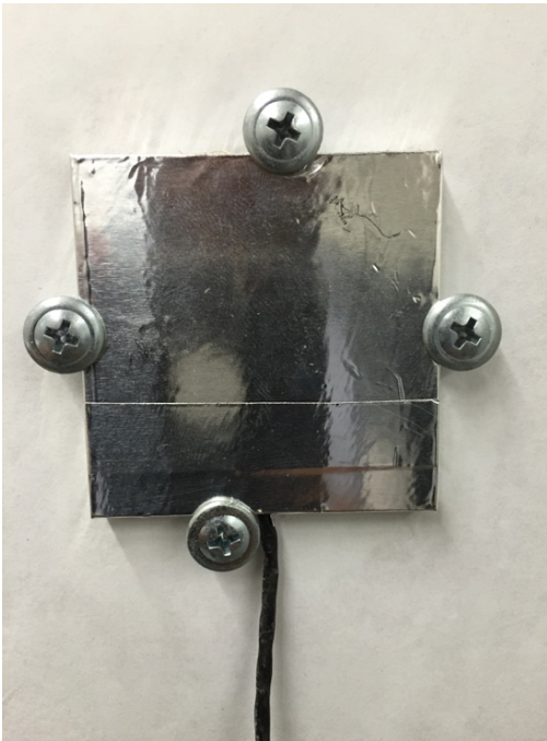
Figure 3.14 Heat Flux Meter Covered with Aluminum Foil
