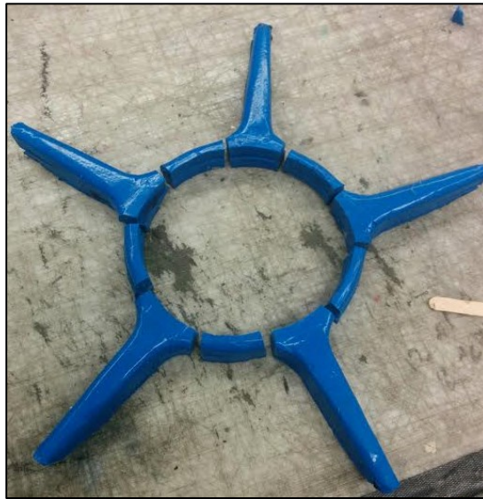
Figure 6.2: RTV rubber tooling
