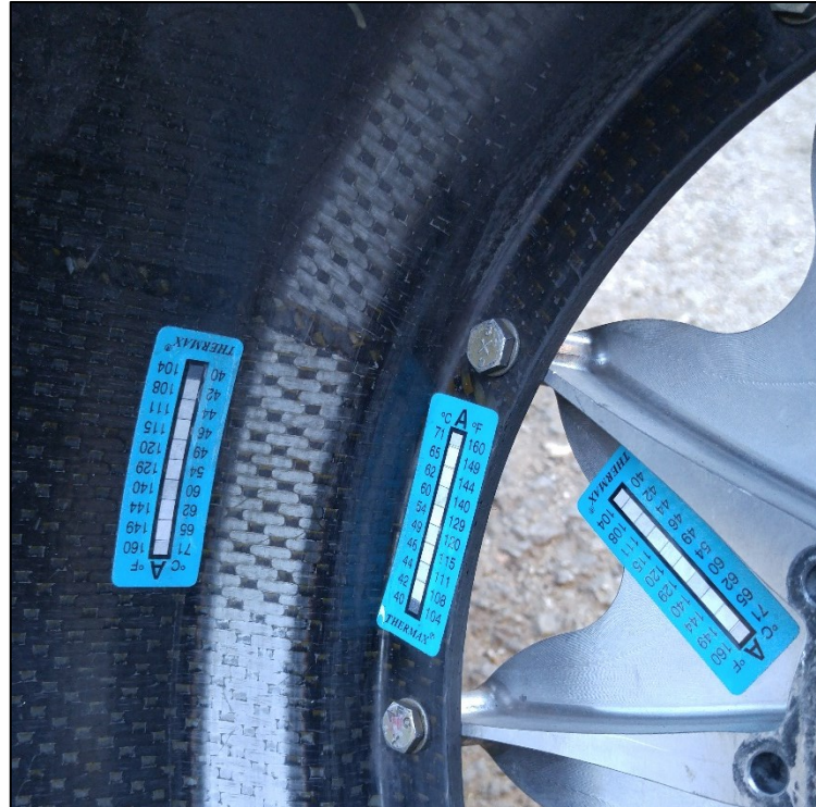
Figure 7.3: Temperature indicating strips on rim
