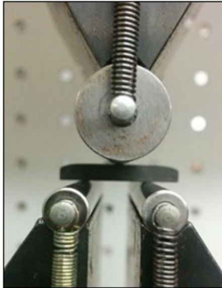
Figure 4.3: Short beam test setup
