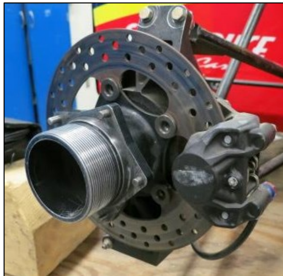
Figure 3.2: Components packaged inside of wheel
