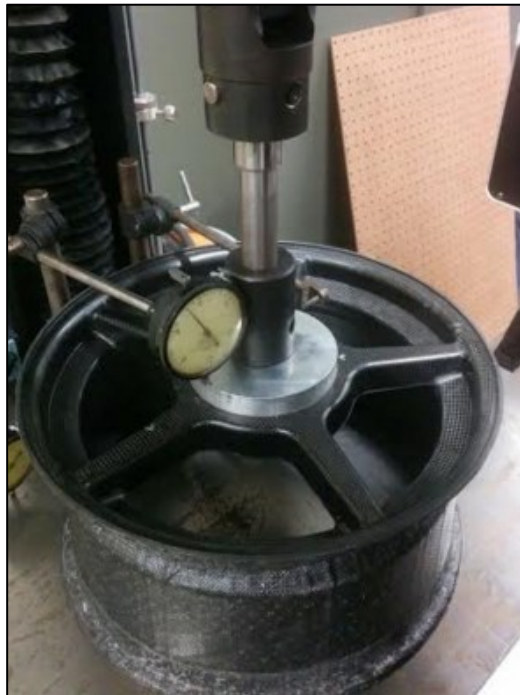
Figure 7.1: Rim displacement test setup
