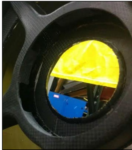
Figure 3.5: Hollow composite wheel spokes
