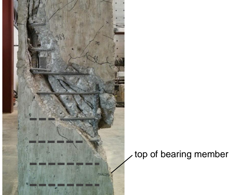
Figure 7.13 Cracks confined by effective confining reinforcement (specimen 11-5-F3.8-6#3-i-2.5-3-12)
