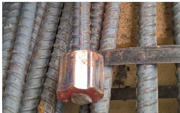
Figure 2.1 Headed bars (a) No. 8 bars (left to right: cold-swaged threaded coupling sleeve, friction-forged, taper-threaded, and cold-swaged), (b) No. 5 (two on left) and No. 11 (two on right) friction-forged bars, (c) No. 11 cold-swaged bars (left one with threaded coupling sleeve), (d) No. 6 cold-swaged bars
