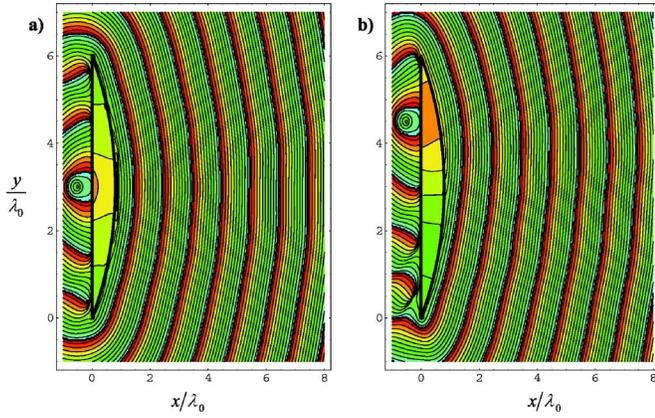
FIG. 15. (Color online) Phase of the magnetic-field distribution when a point source illuminates an ENZ convex lens with  $\epsilon_s = 0.01\epsilon_0$  and radius of curvature of  $6\lambda_0$ . (a) Line source positioned at  $(-0.5, 3.0)\lambda_0$ . (b) Line source positioned at  $(-0.5, 4.5)\lambda_0$ . The color scale is the same as in Fig. 12.
