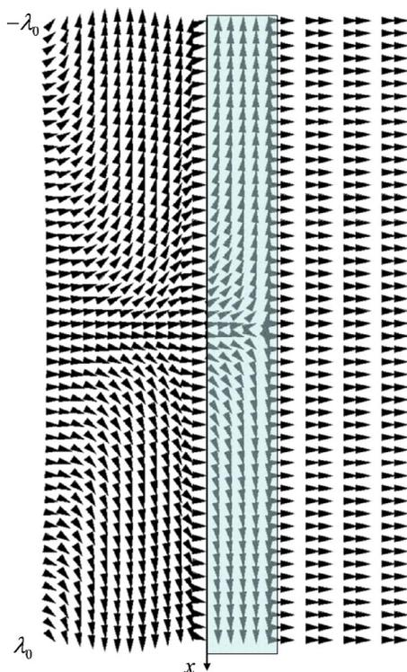
FIG. 5. (Color online) Power flow (real part of the Poynting vector) for a source placed at distance  $d_{source}=2\lambda_0$  from the entrance side of a slab with  $\epsilon_s=10^{-4}\epsilon_0$  and  $d_{slab}=\lambda_0/5$ .
