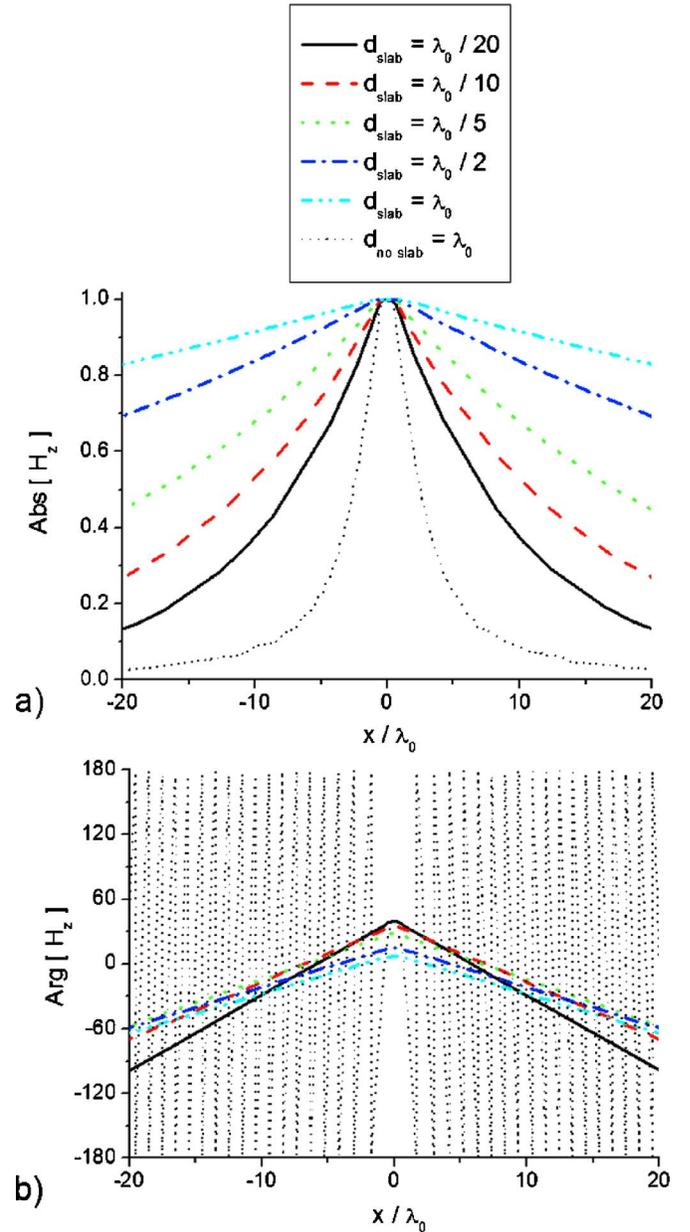
FIG. 4. (Color online) (a) Normalized amplitude and (b) phase distributions at the exit face for an infinite magnetic line current placed at distance  $d_{source} = \lambda_0$  from the entrance side of an ENZ slab with  $\varepsilon_s = 10^{-4} \varepsilon_0$  for different thicknesses  $d_{slab}$ .
