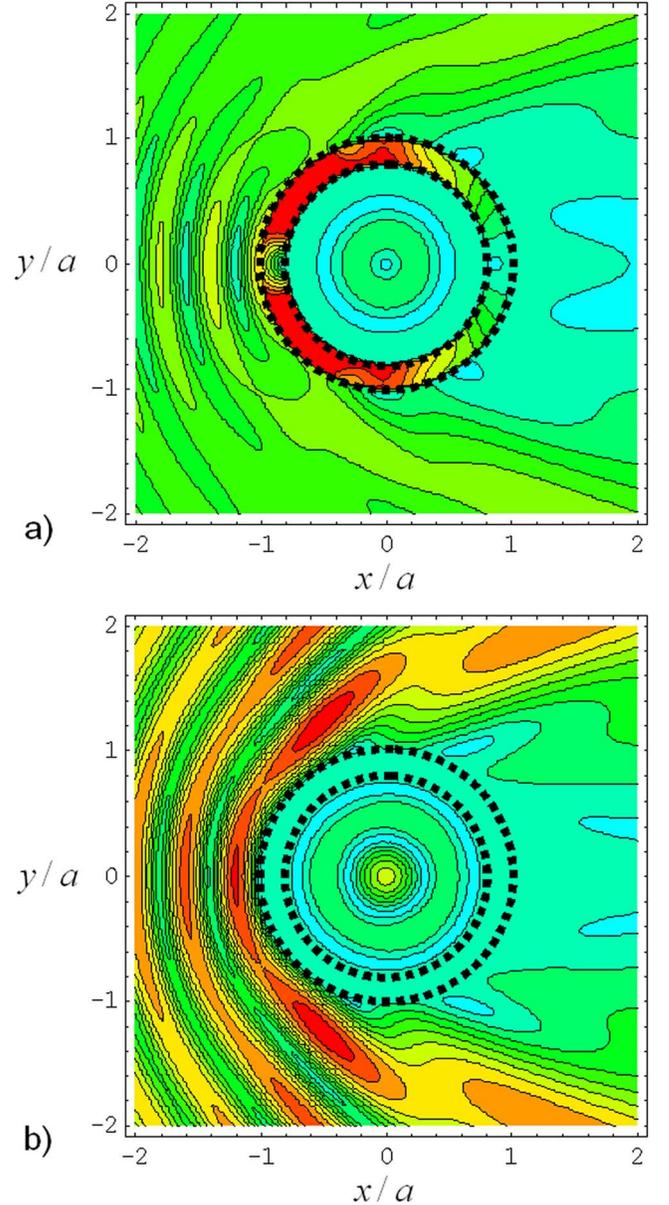
FIG. 10. (Color online) Electric- (a) and magnetic- (b) field distributions for a TM plane wave traveling along  $x$  and impinging on the cylindrical ENZ shell of Fig. 8 with  $a_c = \lambda_0$ ,  $a = a_c/0.8$ , and  $\varepsilon_s = 10^{-3}\varepsilon_0$ . Brighter (darker in gray scale) colors correspond to higher amplitudes of the field.
