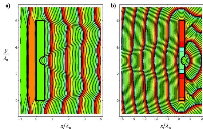
FIG. 18. (Color online) Phase of the magnetic field distribution when (a) a plane wave impinges from the negative  $x$  direction and (b) a point source is positioned at  $(0.5, 3.0)\lambda_0$ , in both cases illuminating a 2D ENZ planar slab with  $\epsilon_s = 0.01\epsilon_0$  with a small semicylindrical cavity carved on its exit face with radius  $R = 0.3\lambda_0$ . The color scale is the same as in Fig. 12.
