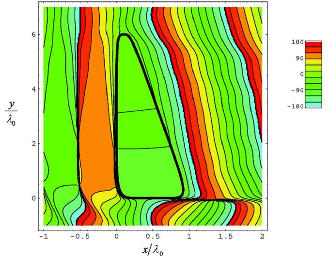
FIG. 12. (Color online) Phase of the magnetic-field distribution (in degrees) when a TM (with magnetic field oriented along  $z$ ) plane wave impinges on a 2D trapezoidal slab with  $\epsilon_s = 0.01\epsilon_0$ .
