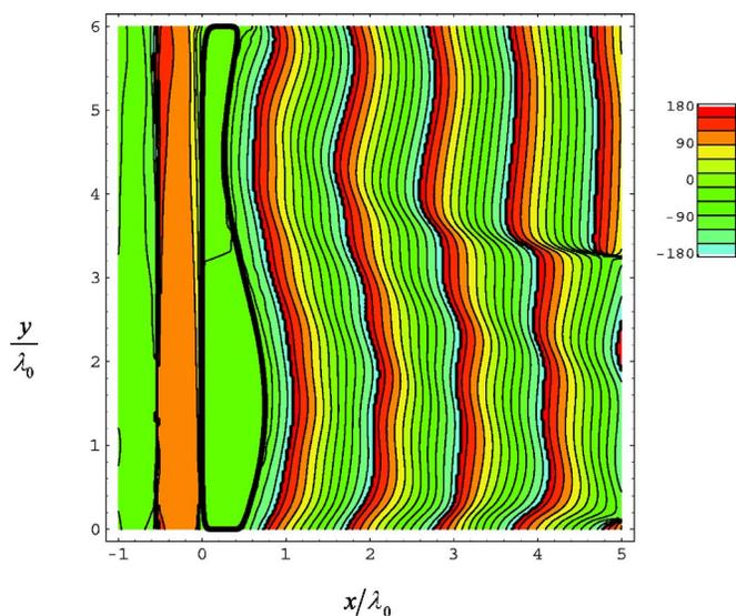
FIG. 13. (Color online) Phase of the magnetic-field distribution when a plane wave illuminates a 2D cylindrical object with  $\epsilon_s = 0.01\epsilon_0$  and arbitrarily shaped output interface.
