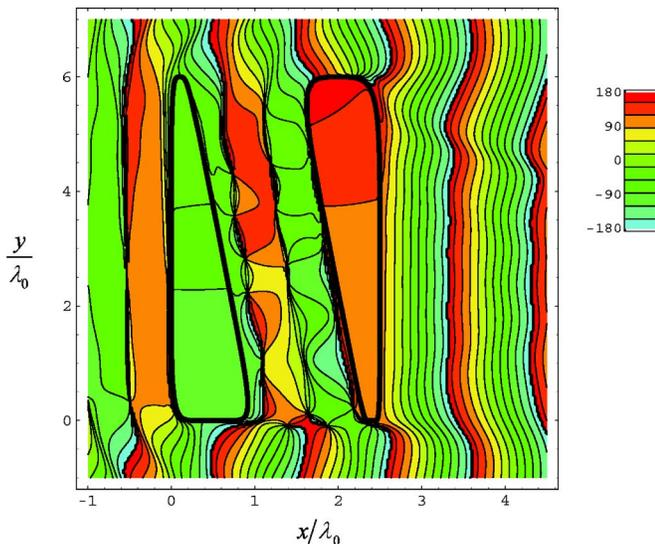
FIG. 16. (Color online) Phase of the magnetic-field distribution when a plane wave (propagating along the positive  $x$  direction) illuminates two complementary ENZ lenses with  $\epsilon_s = 0.01\epsilon_0$ .
