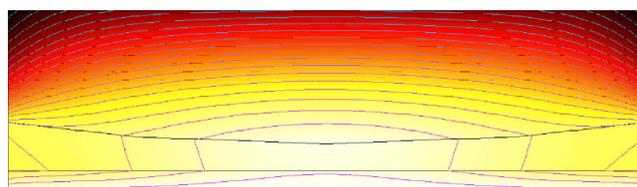
FIG. 7. (Color online) Magnetic-field distribution induced by a plane wave incident on a 2D ENZ slab with concave exit face. The slab width is  $1.2\lambda_0$  and it is assumed to be made of realistic silver with permittivity  $\epsilon_s=0.016+i0.42$  at the frequency for which  $\lambda_0=325$  nm, following experimental data (Ref. 11). Brighter (lighter in gray scale) colors correspond to higher amplitude values of the magnetic field. The dark lines represent equiphase fronts.
