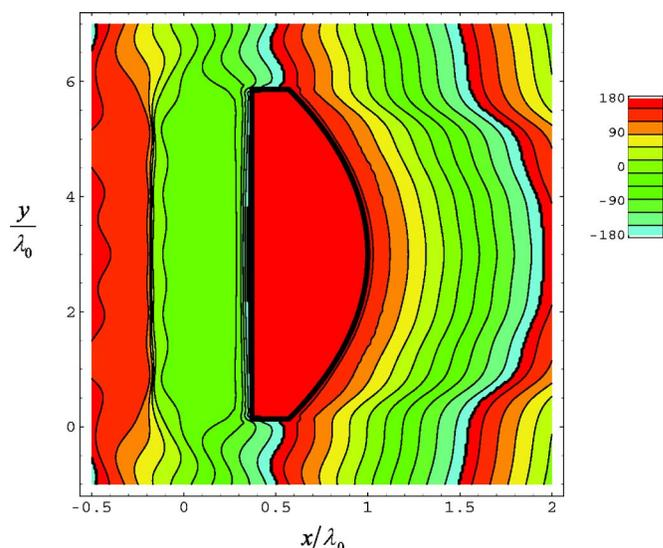
FIG. 19. (Color online) Phase of the magnetic-field distribution when a plane wave (propagating along the positive  $x$  direction) illuminates a 2D lens with  $\epsilon_s = 0.01\epsilon_0$  designed to obtain a prescribed phase front at the output plane.
