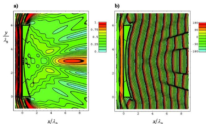
FIG. 14. (Color online) (a) Normalized amplitude and (b) phase of the magnetic-field distribution when a plane wave illuminates a 2D concave lens with  $\epsilon_s = 0.01\epsilon_0$  and radius of curvature of  $6\lambda_0$ .
