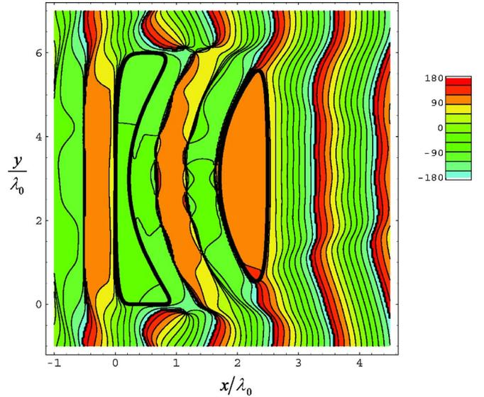
FIG. 17. (Color online) Phase of the magnetic-field distribution when a plane wave (propagating along the positive  $x$  direction) illuminates two complementary ENZ lenses with  $\epsilon_s = 0.01\epsilon_0$ . The first object has a concave exit face and the second object has a convex entrance face.
