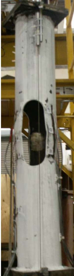
FIG. H1 - PEAK DEFORMATION UNDER TENSION LOAD; LOAD STEP #11 LAST CYCLE.
