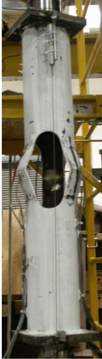
FIG. G2 - PEAK DEFORMATION UNDER COMPRESSION LOAD; LOAD STEP #10 LAST CYCLE.
