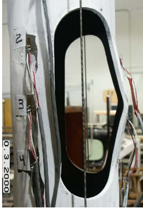
FIG. D2 – FIRST ARM THAT BUCKLED, PEAK COMPRESSION DISPLACEMENT LOAD STEP #6.
