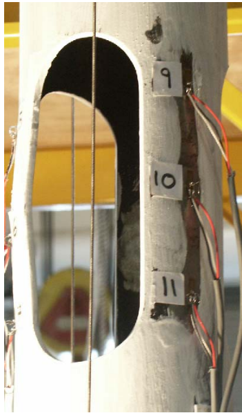
FIG. B1- INITIAL BUCKLING DEFORMATION AT ONE ARM; LOAD STEP #2 FIRST CYCLE.
