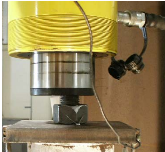
FIG. B2 - INITIAL ECCENTRICITY.
