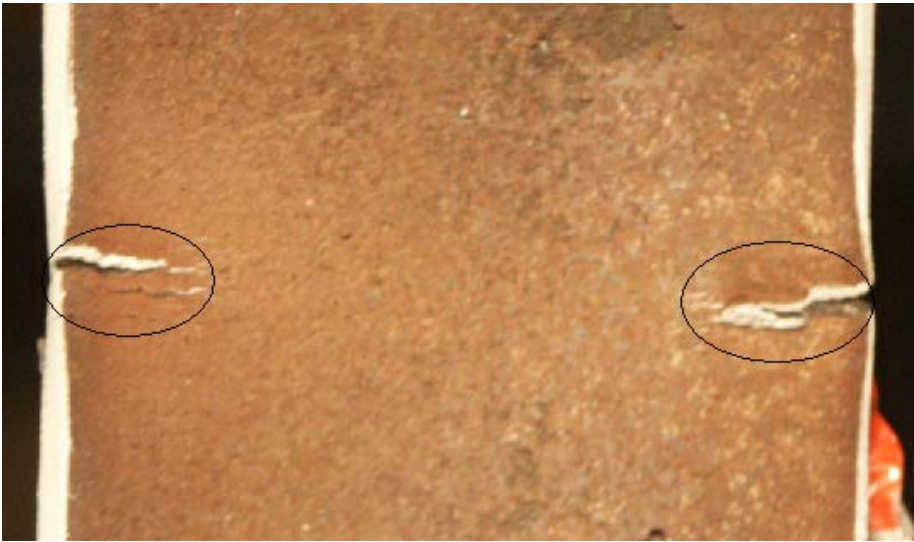
FIG. I4 – FATIGUE FAILURE CLOSE-UP FROM INSIDE, LOAD STEP #12, FIRST CYCLE.
