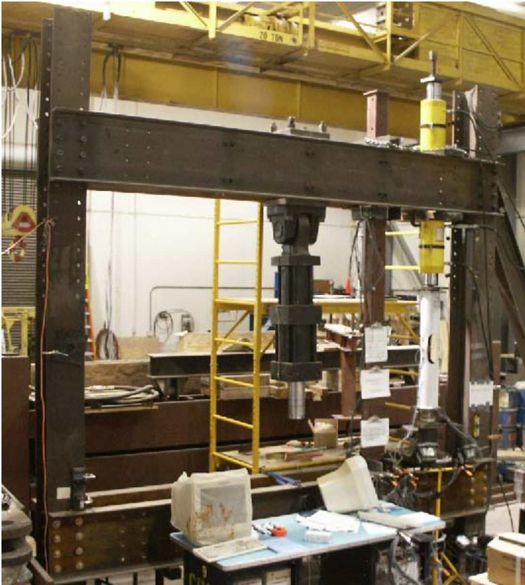
FIG. A1 – TEST SET-UP PHOTO; REACTING FRAME.
