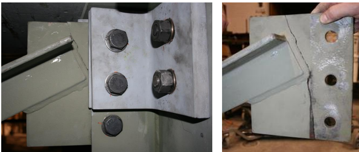
Figure 11: North cross frame failure during Trial 4N.
