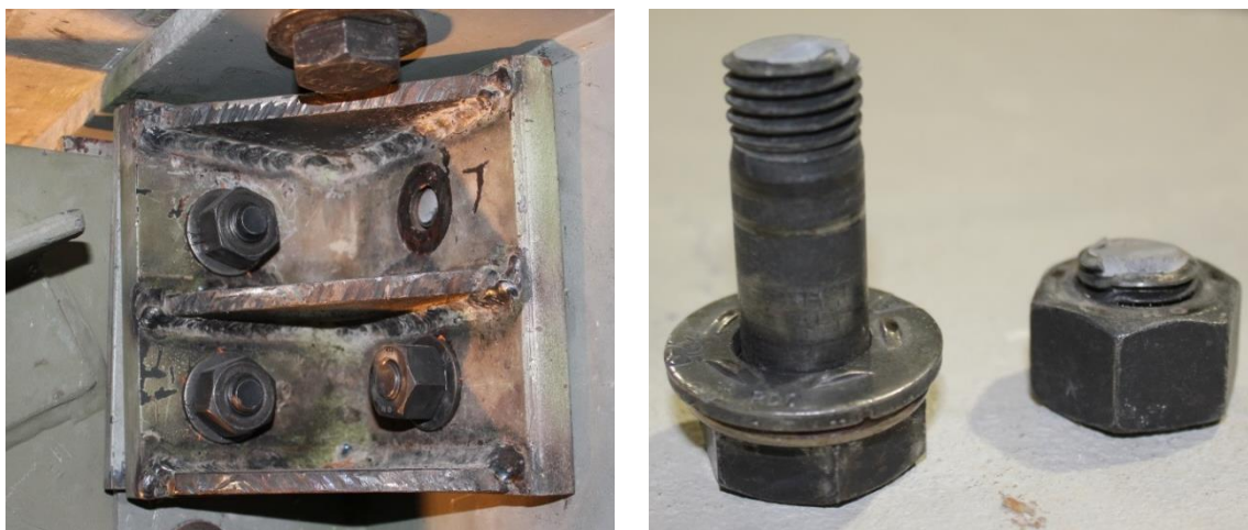
Figure 15: Broken bolt at the end of Trial 2.3N.
