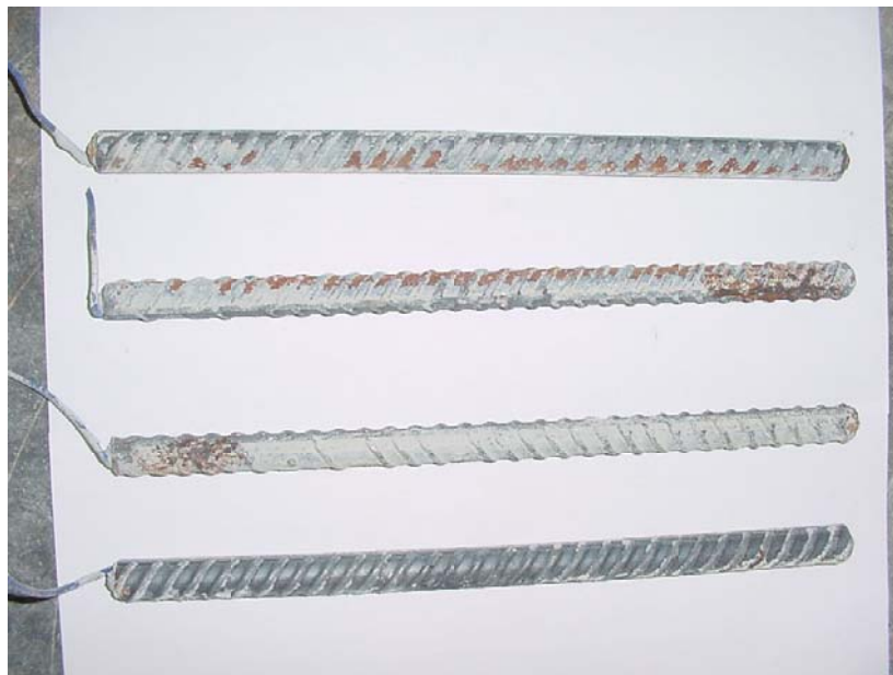
Figure 3.34 – Corrosion products on bottom bars of specimen SE-CRPT1-3
