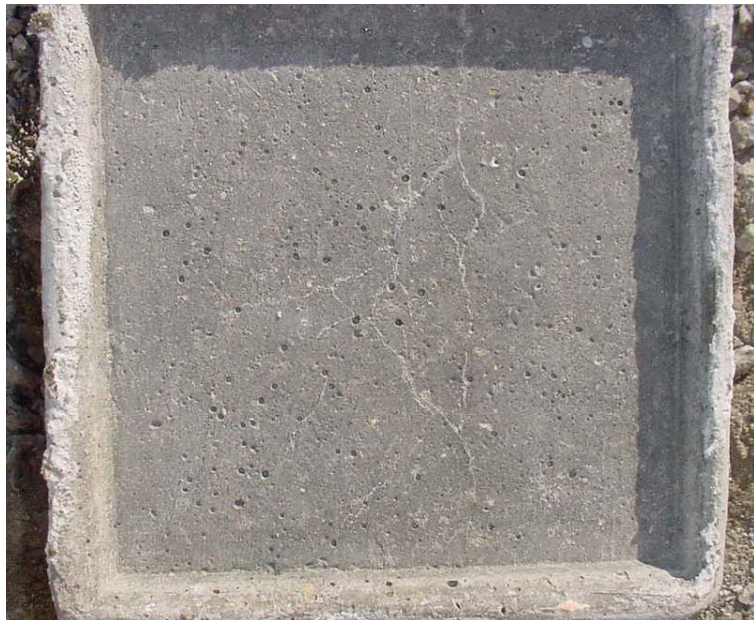
Figure 3.30 – Thin cracks on specimen SE-CRPT1/N-3
