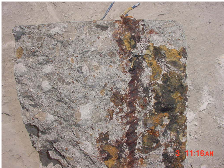
Figure 3.32 – Corrosion products on top bar of specimen SE-CRPT2-1
