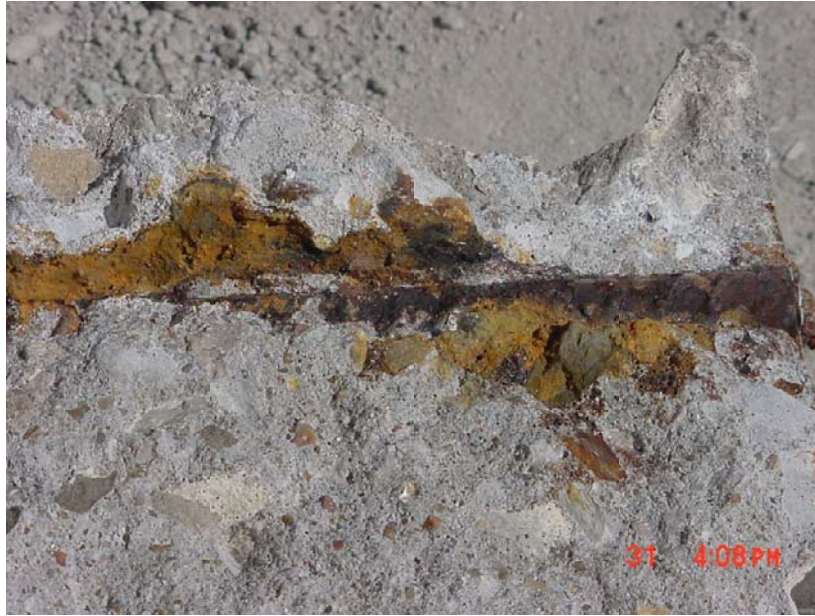
Figure 3.33 – Corrosion products on top bar of specimen SE-CRT-1 (side view of specimen).
