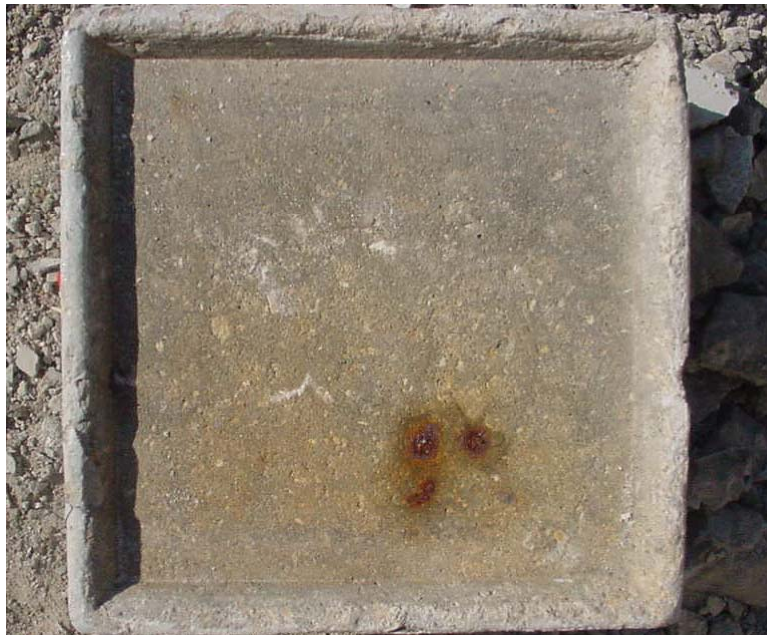
Figure 3.29 – Rust stains on surface of specimen SE-CRPT2-1
