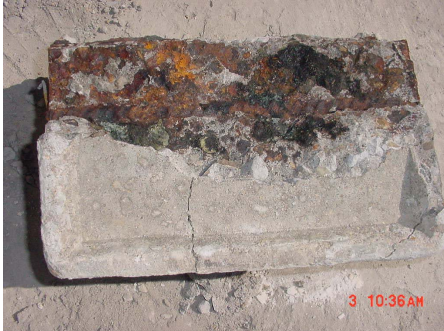
Figure 3.31 – Corrosion products on top bar of specimen SE-N-3
