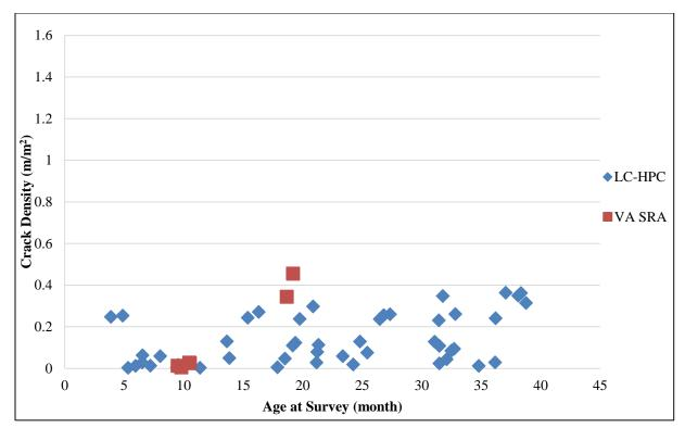
Figure 11: Crack densities of LC-HPC decks and SRA decks versus bridge age
