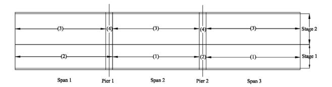
Figure 9A: Construction Sequence of VA-9
