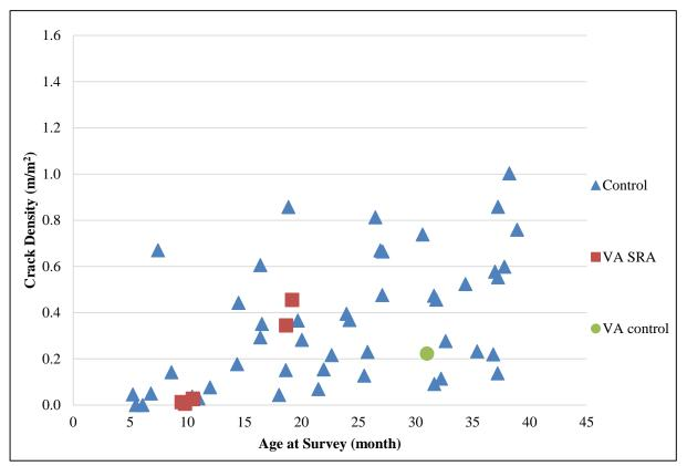
Figure 10: Crack densities of control decks and SRA decks versus bridge age
