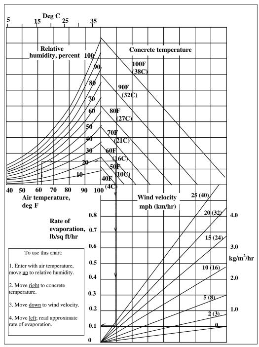
FIGURE 710-1: STANDARD PRACTICE FOR CURING CONCRETE
