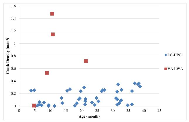
Figure 13: Crack densities of Virginia bridge decks using lightweight aggregate and LC-HPC decks versus deck age
