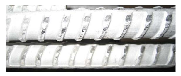
**Figure 1a:** Damage to deformations on straightened XM-28 bars from the straightening process.
