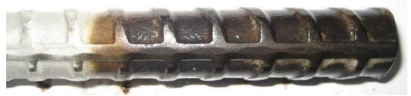
**Figure 16b:** Straightened XM-28 stainless steel from producer A after testing; specimen XM28s-5. Anode bar with severe discoloration.
