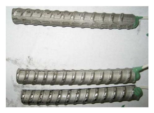
**Figure 13:** Coiled XM-28 stainless steel from producer A after testing; specimen XM28c-2. Anode (top bar) and cathode (bottom bars).
