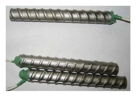
**Figure 18:** XM-28 stainless steel from producer B showing mild discoloration after testing; specimen XM28-1. Anode (top bar) and cathode (bottom bars).
