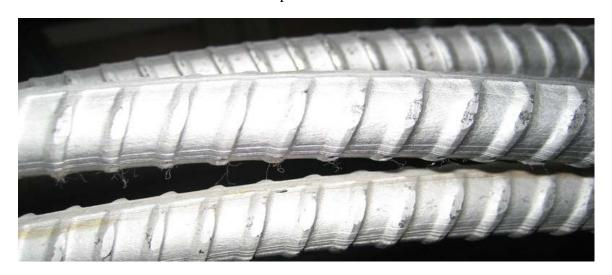
**Figure 1b:** Damage to deformations on coiled XM-28 bars.
