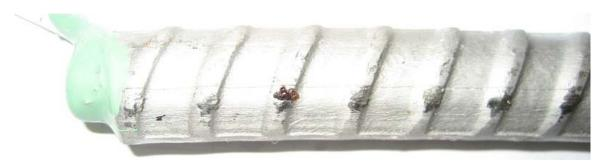
**Figure 14:** Coiled XM-28 stainless steel from producer A after testing; specimen XM28c-1. Anode bar with limited corrosion products at a damage site.
