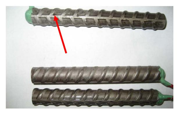
**Figure 19a:** 2205 stainless steel from producer B showing discoloration and corrosion products (arrow) after testing; specimen 2205-1. Anode (top bar) and cathode (bottom bars).
