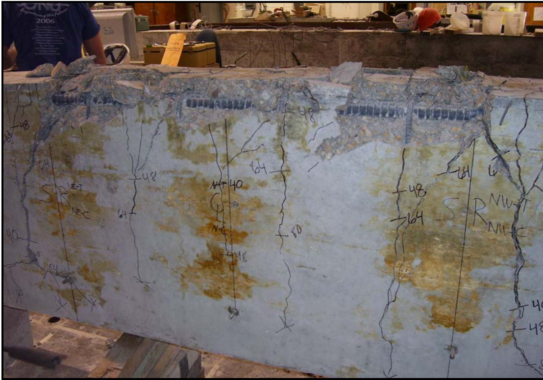
Figure B.10 - Beam 8-5-OC1-1.5 at the conclusion of the test
