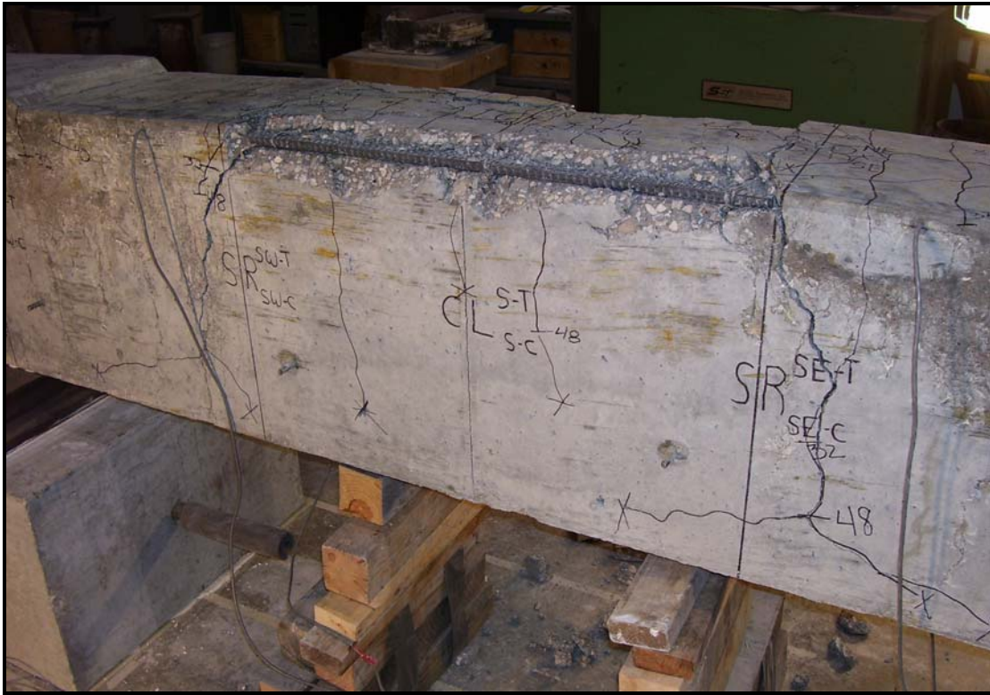
Figure B.3 - Beam 5-5-OC0-3/4 at the conclusion of the test
