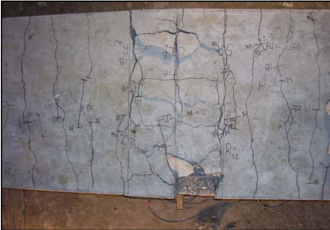
Figure B.6 - Beam 5-5-OC0-2d b at the conclusion of the test, as viewed from above
