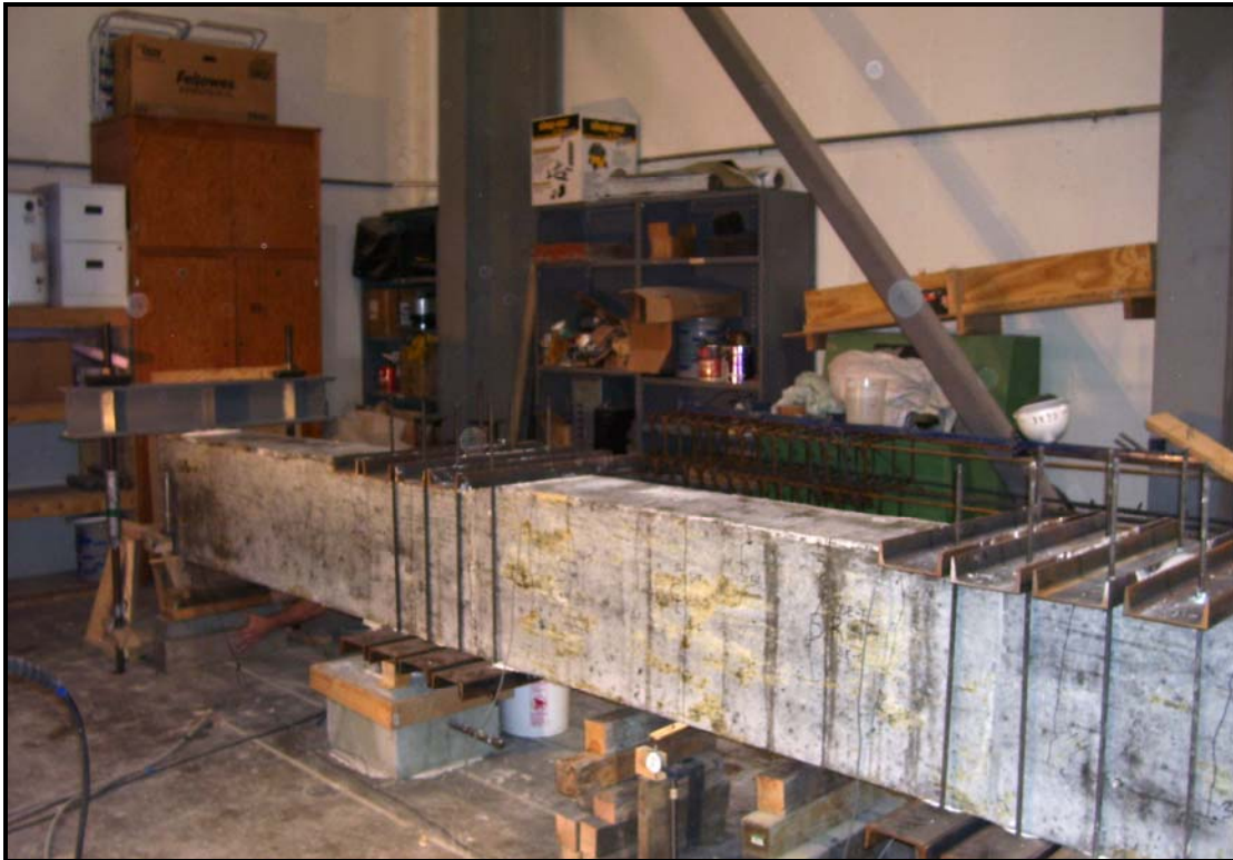
Figure B.24 - External stirrups used on beam 8-8-XC2-2.5
