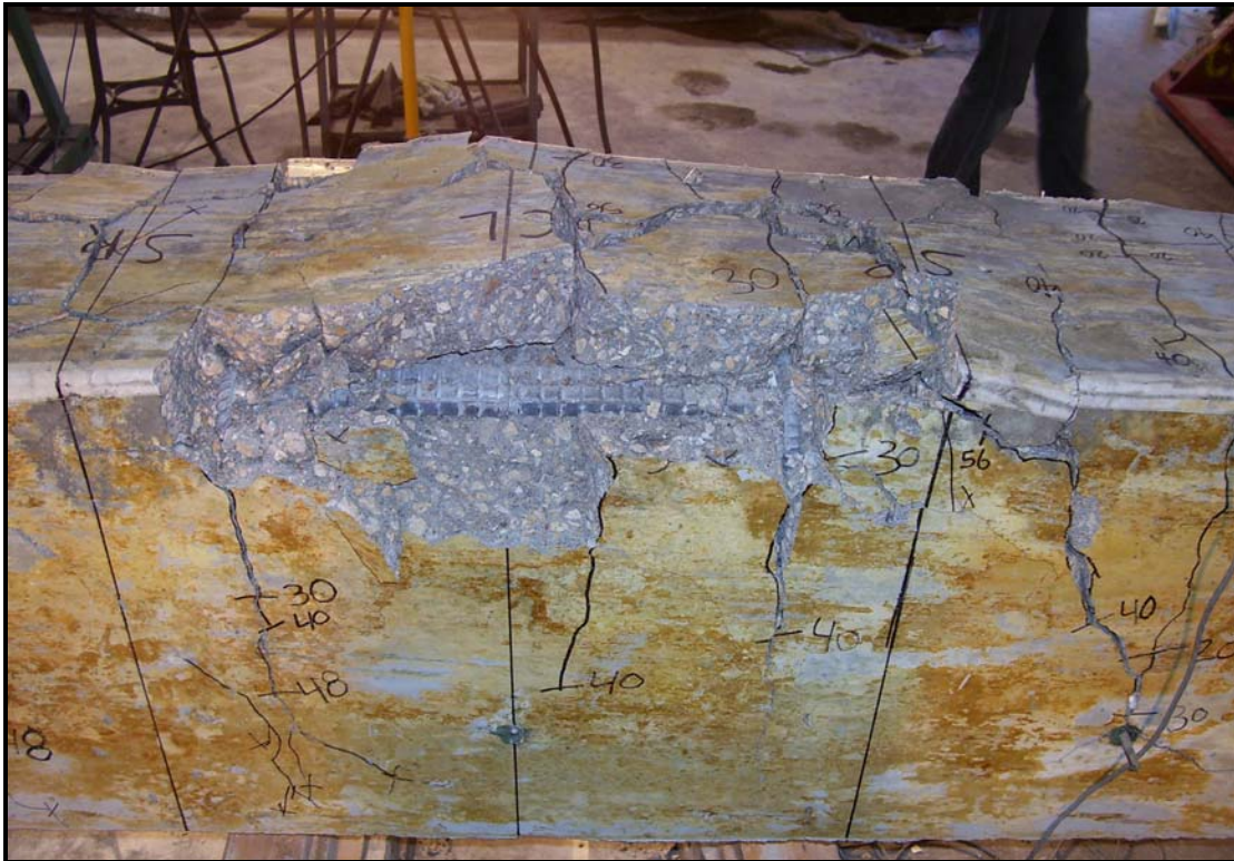
Figure B.22 - Beam 8-8-XC1-2.5 at the conclusion of the test
