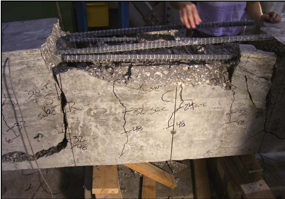
Figure B.21 - Beam 8-8-XC0-2.5 at the conclusion of the test
