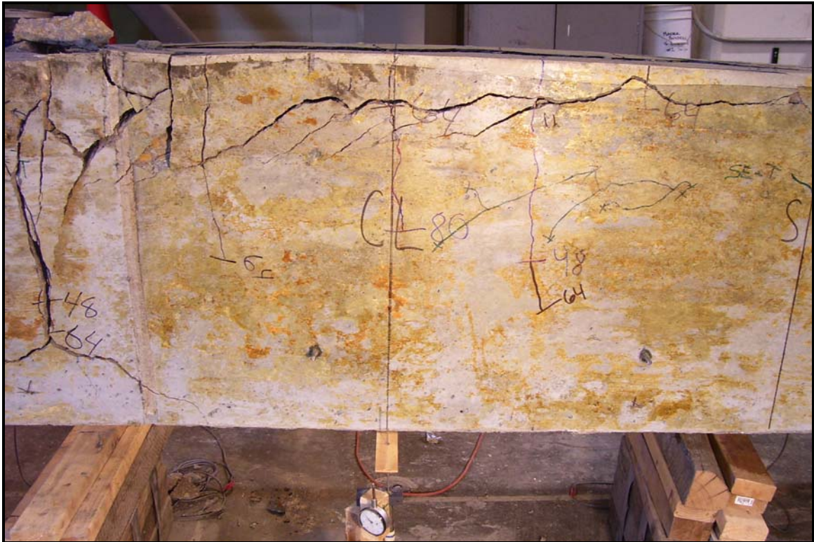
Figure B.26 - Beam 11-8-OC0-2 at the conclusion of the test
