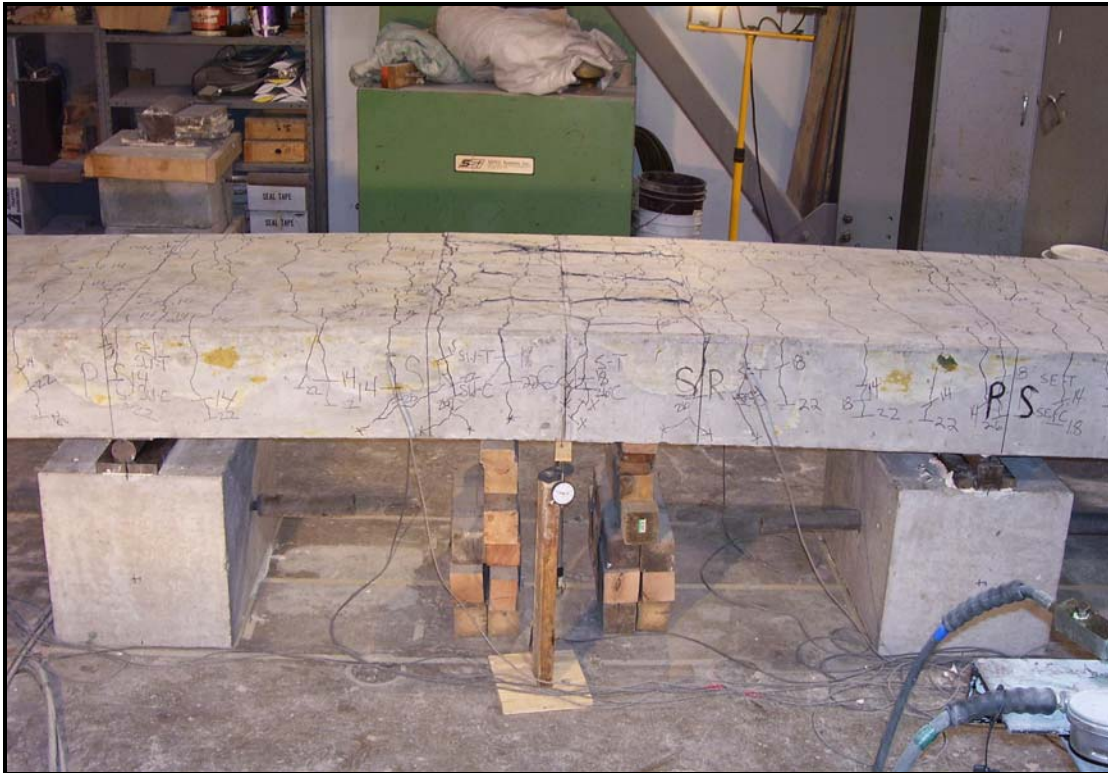
Figure B.7 - Beam 5-5-XC0-2d b at the conclusion of the test
