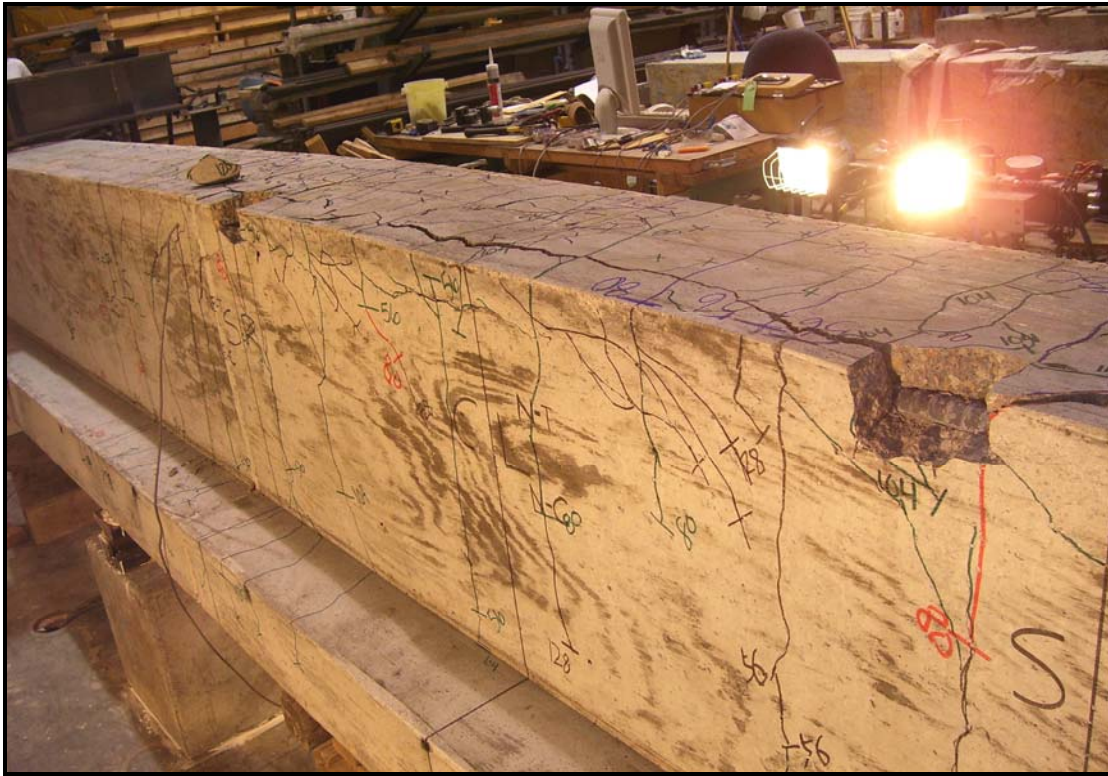
Figure B.15 - Beam 8-5-XC1-1.5 at the conclusion of the test
