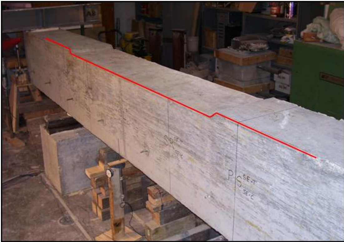
Figure B.1 - Specimen 5-5-XC0-3/4 with the reduced “dog-bone” section
