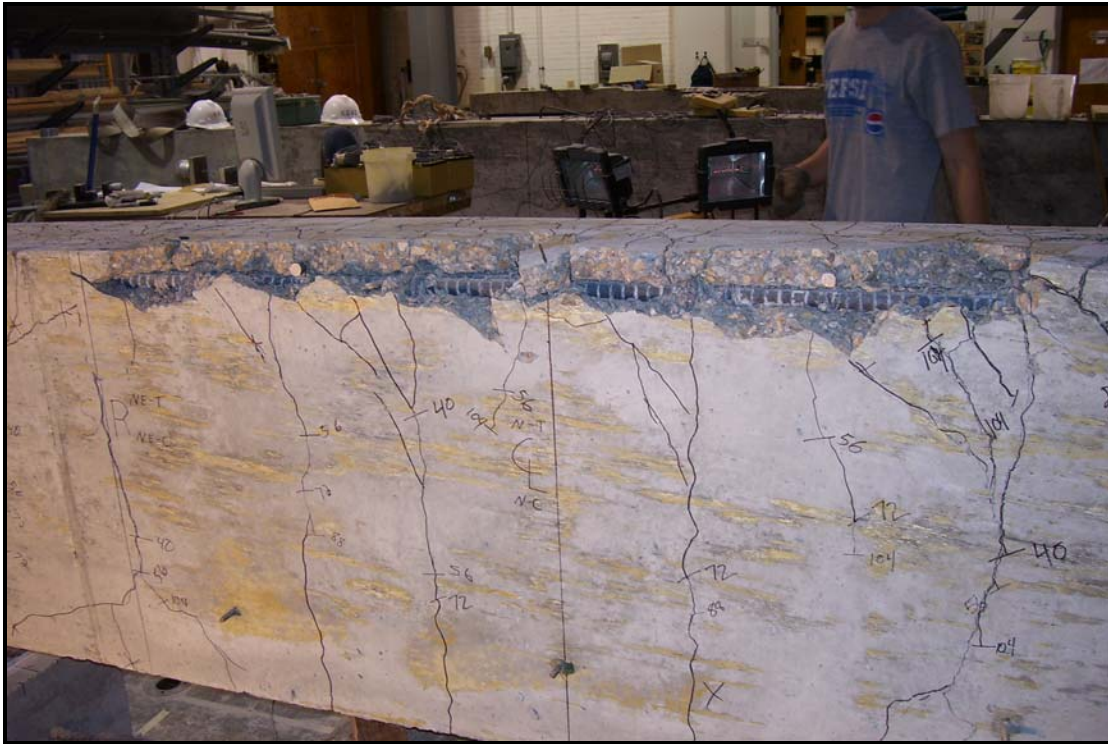
Figure B.14 - Beam 8-5-XC1-1.5 at the conclusion of the test
