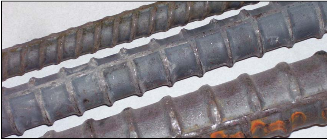
Figure 2.4 - Photograph of No. 5, No. 8, and No. 11 Grade 100 reinforcing steel
