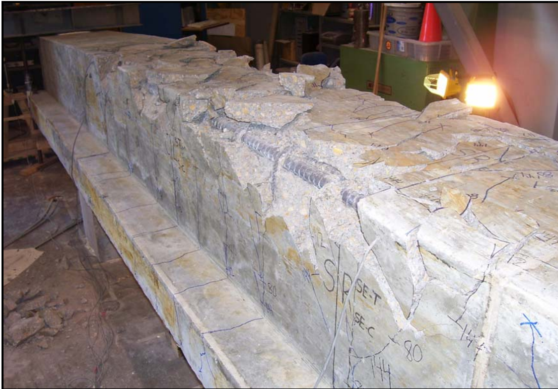
Figure B.32 - Beam 11-8-XC2-2 at the conclusion of the test
