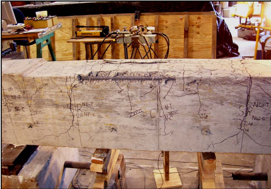
Figure B.4 - Beam 5-5-XC0-3/4 at the conclusion of the test
