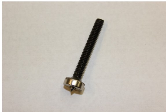
Figure B-7: PACTS tool leg assembly with sharpened steel screw and countersunk magnet.
