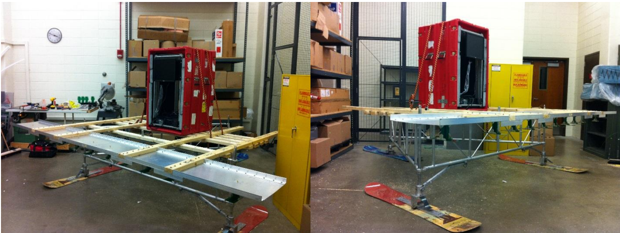
Figure 6. Assembled sled platform with antenna array and radar case.
