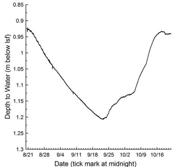
**Figure 7.** Depth to water from land surface recorded at well Ash32 in the ARS from 20 August to 22 October 2004. Well is located in stand of small salt cedar apparently under stress (many of the salt cedar had a yellowish tinge). Butler *et al.* [2005] provide details of well site and a photograph of vegetation (salt cedar in the vicinity of well were last cut at the same time as those in Figure 1; see Figure 1 caption for further details regarding post 21 September increases in water level).
