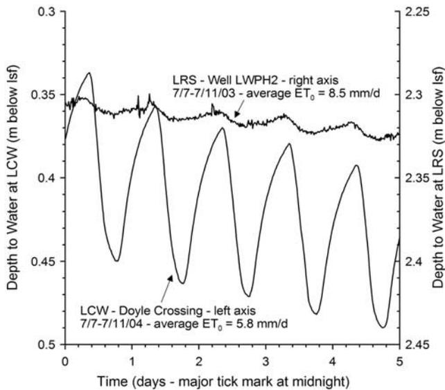
**Figure 11.** Variations in diurnal fluctuations in the water table between wells at the LRS and LCW. Shallow subsurface is primarily coarse sand and gravel at LRS, whereas it is primarily silt at LCW. LRS 7–11 July 2004 data were impacted by high river flows and so are not presented. LCW was not monitored in 2003. Diurnal fluctuations at well LWP2 have the largest amplitude observed in the vegetated riparian zone at the LRS.
