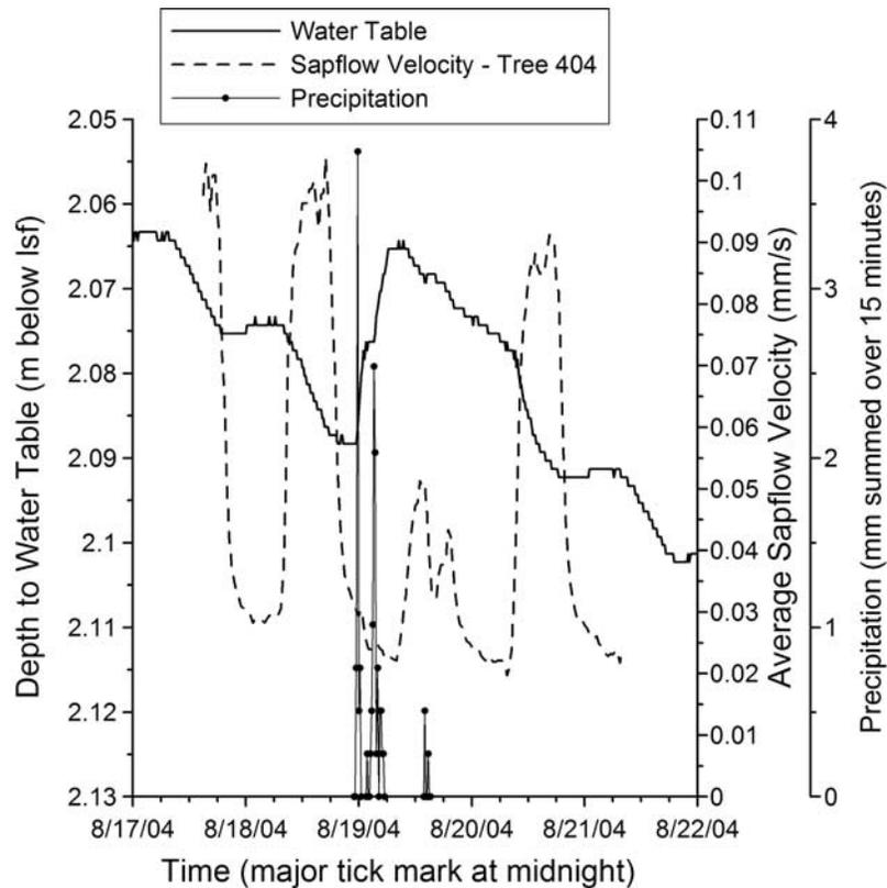
**Figure 3b.** Depth to water table from land surface at well LWP2 in LRS with sap flow velocity and precipitation as in Figure 3a (well located in the center of the riparian zone just west of the river channel (Figure 2)). There was no flow in the Arkansas River at the LRS during this period. The general decline in the water table is caused by plant water use and by pumping in the underlying High Plains aquifer.
