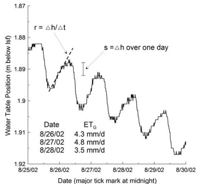
**Figure 12.** Example application of the White method using late August 2002 water level data from well LWP3 at the LRS. There was no flow in the Arkansas River and little precipitation (0.003 and 0.002 m for 26 and 27 August, respectively) at the LRS during this period.
