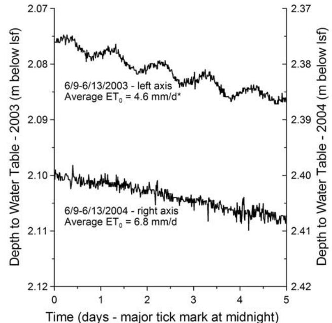
**Figure 9.** Variations in water table position at well LWPH3 in the LRS for early June of 2003 and 2004. Asterisk indicates no 9 June 2003  $ET_0$  estimate; break in trend in final day of 2003 data coincides with a reduction in  $ET_0$  to 2.9 mm/d. There was no flow in the Arkansas River and little precipitation (0.002 m on 9 June 2004) at the LRS during these periods. The general decline in the water table is caused by plant water use and by pumping in the underlying High Plains aquifer.
