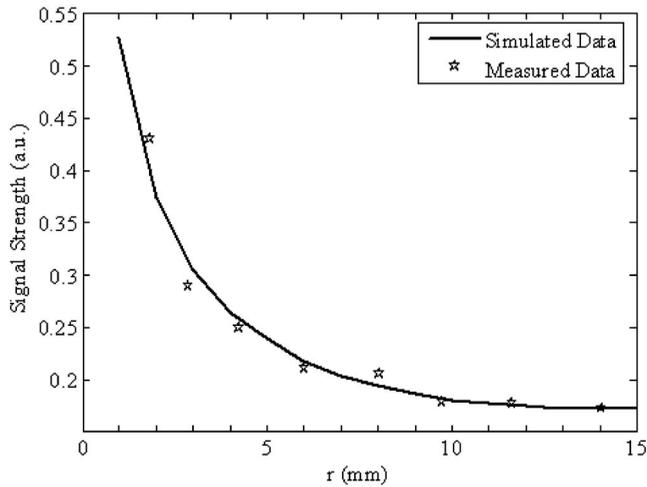
**Fig. 3** The signal strength of a point on a line target as a function of the distance  $r$  between the scan center and the center of the virtual point detector. The solid line represents the simulated data, and the asterisks represent the measured data.
