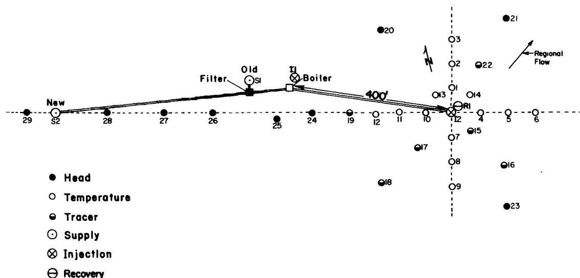
Fig. 2. Top view of the well field at the Mobile site showing the different types of wells.
