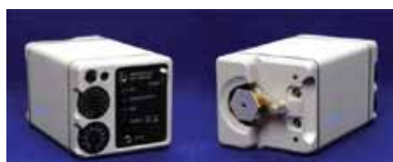
Figure 3. A peristaltic pump was connected to the perfusion chamber at a flow rate of 10 \mu L/sec to flow fluid through the chamber.
