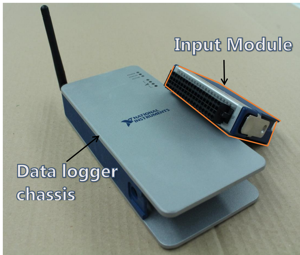
Fig. 18. Data logger with measurement module.
