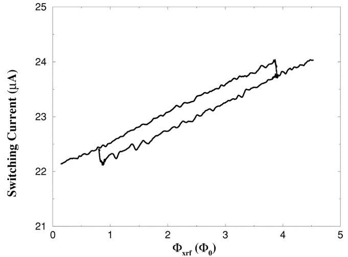
Fig. 3. The rf SQUID's hysteresis loop detected by the dc SQUID switch at 4.2 K. The higher (lower) branch of the loop corresponds to the  $|0\rangle$  ( $|1\rangle$ ) qubit state.
