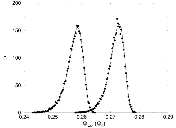
Fig. 5. The flux distributions of the dc SQUID detector at  $T = 1.4$  K. Since the detector was flux biased on the negative-slope side of  $I_S(\Phi_{x\text{dc}})$  the left (right) one corresponds to the qubit in state  $|0\rangle$  ( $|1\rangle$ ). These distributions result in a single-shot readout efficiency of about  $98.8\%$ .
