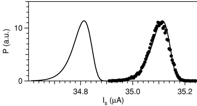
Fig. 4. Switching current distribution of a dc SQUID detector measured at  $T = 10$  mK (solid dots). The solid lines are calculated from MQT theory. The distribution on the left is separated by  $0.3 \mu\text{A}$  from the one on the right. The overlapping part of the two distributions, when normalized, is less than  $10^{-4}$ .
