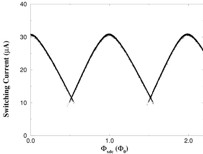
Fig. 2. The flux modulation of the switching current of the dc SQUID at  $T = 1.55$  K.
