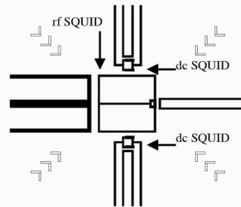
Fig. 1. Top: the equivalent circuit of a flux qubit coupled to a dc SQUID readout device through mutual inductance  $M$ . Bottom: the layout of a gradiometer flux qubit inductively coupled to two unshunted dc SQUID detectors.
