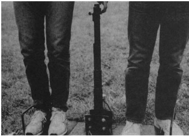
FIG. 5. Photograph of downhole configuration of the .50-caliber rifle.
