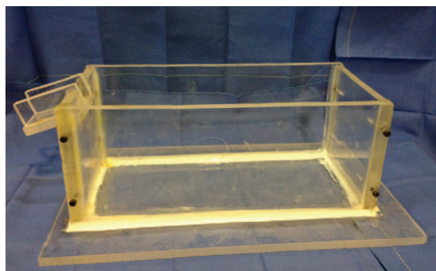
Figure 1. A Plexiglas box was constructed to conduct volumetric measurement of the foot by water displacement.
