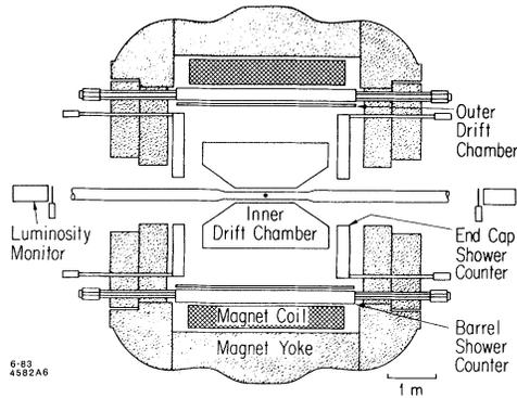
FIG. 1. The high resolution spectrometer (HRS).
