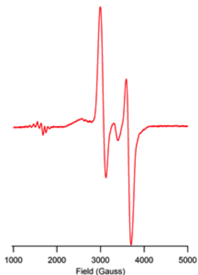
Figure 3.7: EPR spectrum of [\text{Cu}_2(\text{PyEtAm}_{\text{H-4}})]
