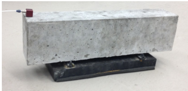
Figure 2.6 Impact resonance test – specimen setup
