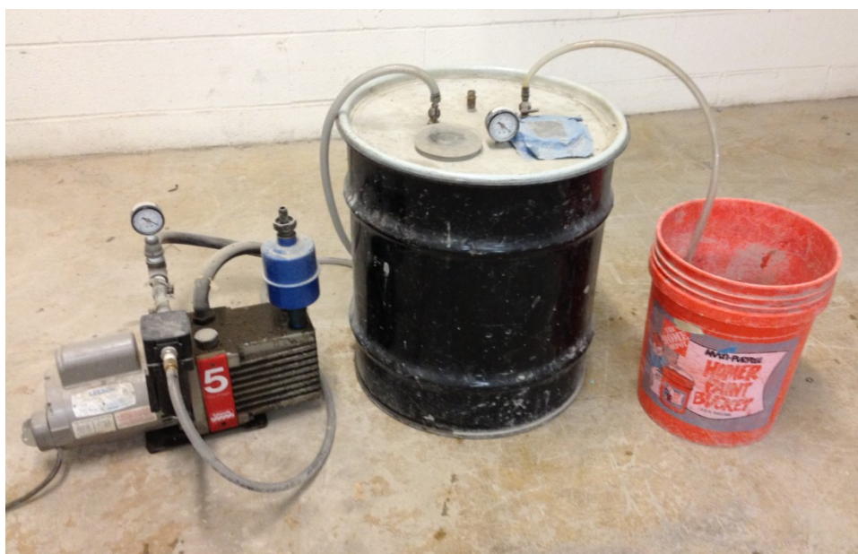
Figure 2.1 Vacuum pre-wetting equipment
