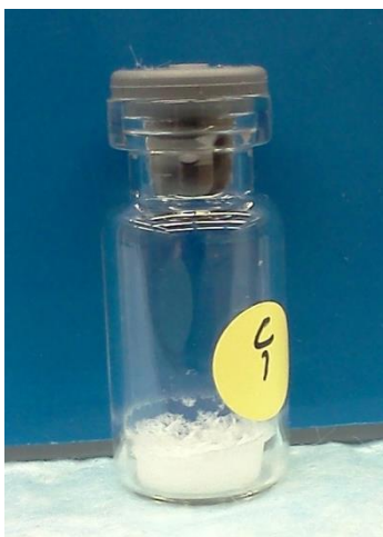
Figure 2.2 Vial containing lyophilized protein formulation The resulting formulation is an amorphous solid.
