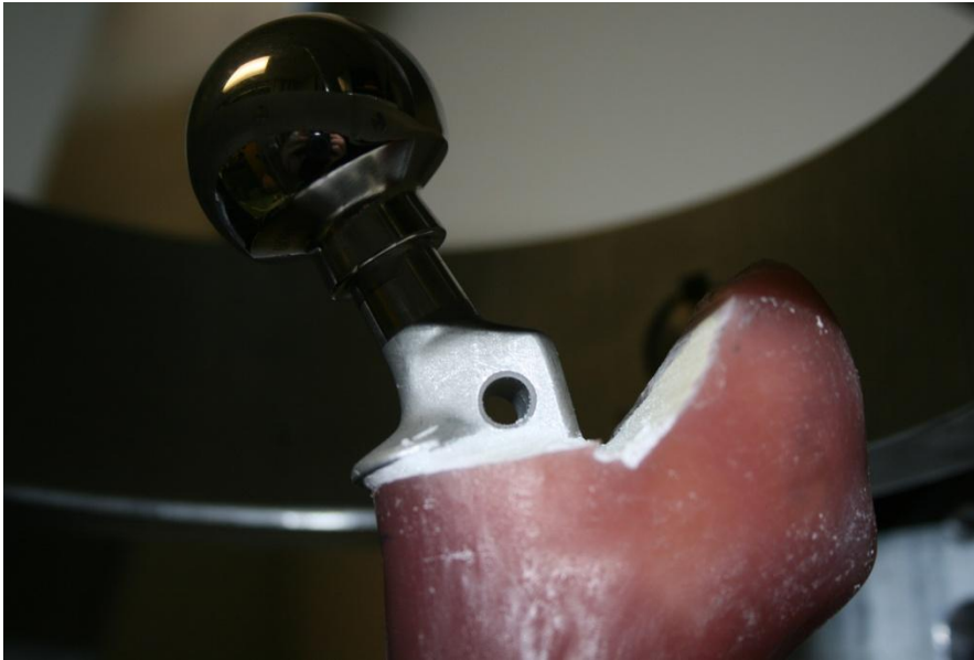
Figure 2. Image of the proximal end of a 3 rd generation saw bone with a cemented femoral stem inserted.
