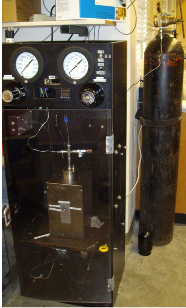
Figure 61 Fluid loss cell placed inside a pressure control cabinet supplied with a nitrogen tank
