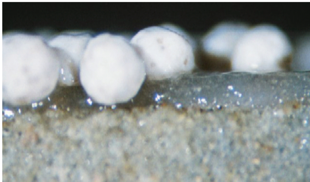
Figure 50 Filter cake build up of 35 ppt Zr X-linked CMHPG (Palisch et al.) [8]
