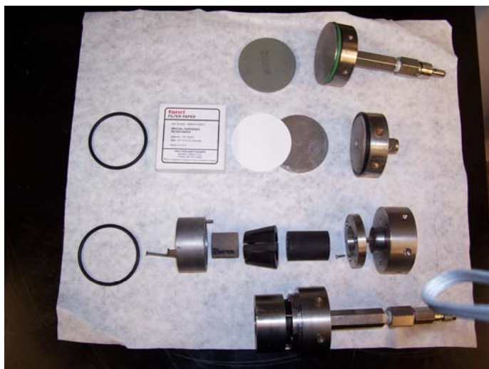
Figure 64 Various endcap assemblies for short cell. The assembled core endcap is shown at the bottom of the picture [94] The top two are the endcap used for disk or filter paper supported by a disk. The third and fourth from the top show the assembly of the setup for cores. (photo by Richard Hutchins, used by permission) [94]
