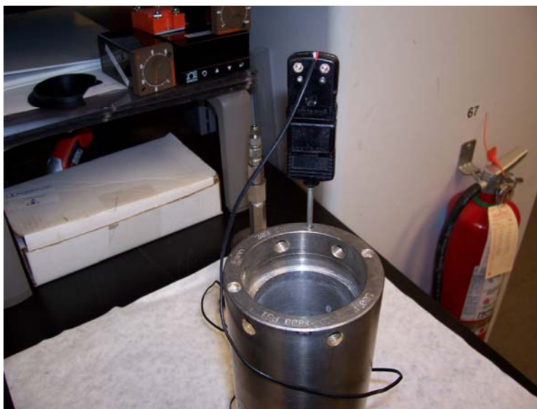
Figure 63 Fluid loss cell with thermocouple inserted (photo by Richard Hutchins, used by permission) 1941
