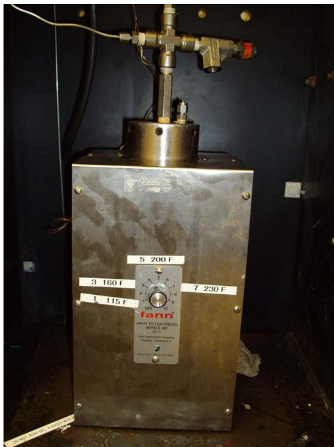
Figure 62 Cell heater with thermocouple inserted inside for preheating. A thermocouple is placed inside the heating jacket to control its temperature.
