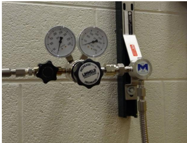
Figure 23. Fuel additive system: Matheson Gas series 3210 Two-Stage stainless steel high-purity regulator.
