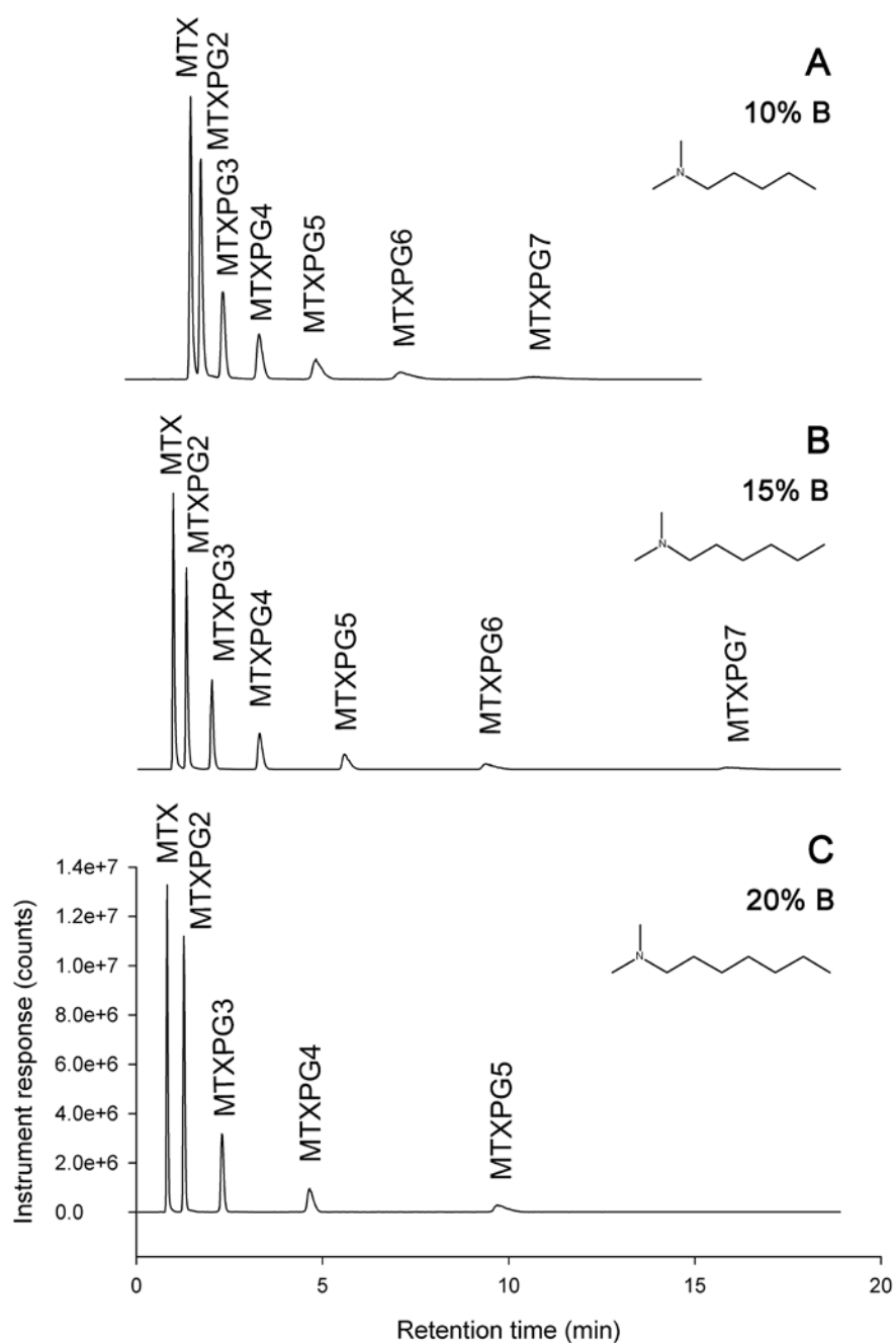
Figure 35. Isocratic separations of aqueous mixtures of MTXPGs demonstrating selectivity differences between the ion pair reagents. Each chromatogram is obtained with the IP concentration fixed at 5 mM. (A) Separation obtained with DMPA, (B) Separation obtained with DMHA, (C) Separation obtained with DMHPA.
