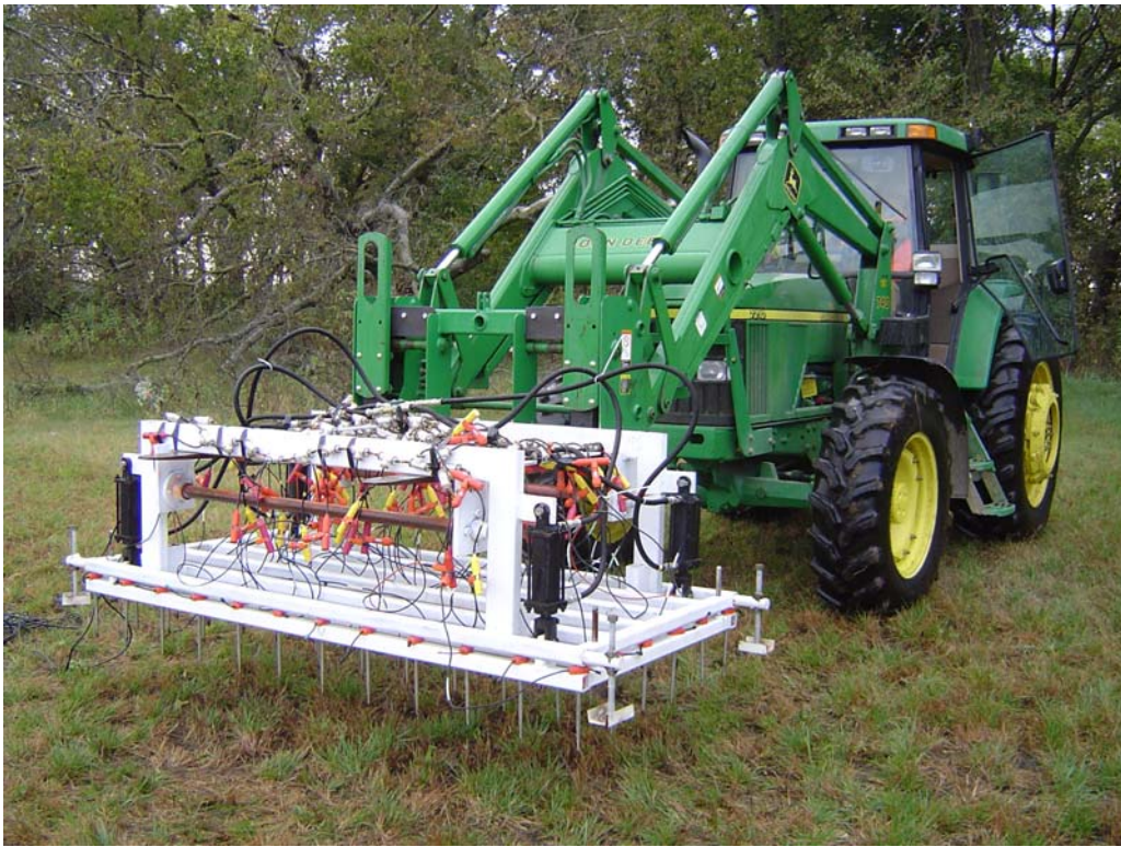
Figure 4.1. Photo of the pilot array, capable of planting 72 geophones simultaneously using the front-end loader of a tractor.
