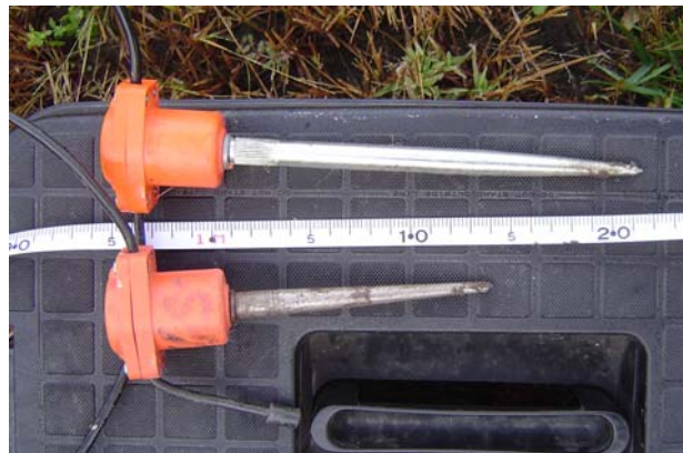
Figure 4.5. Photo illustrating the difference in spike length for 3DAJ-planted geophones (top) and hand-planted geophones (bottom).
