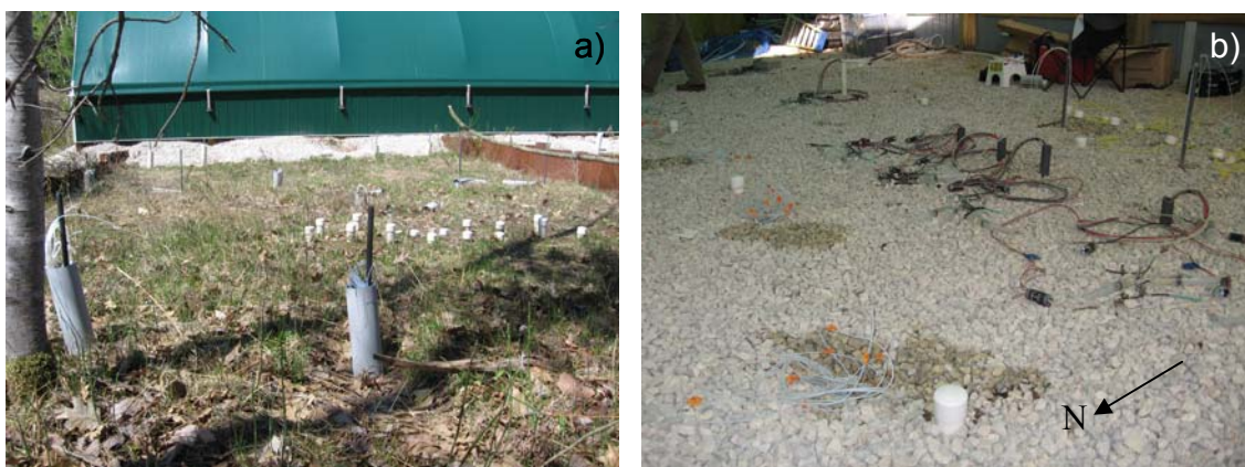
Figure 1.4: Location of the 15 source release wells that introduced the petroleum hydrocarbon into the aquifer (a). Note the sheet piling to the right and left of the 2” white well heads. Three rows of multilevel sampling wells (grey) can be noted outside the green structure. The green structure is ~ 13 m directly down-gradient and due north of the release wells. Inside the green structure is the primary monitoring area for this study (b). Five PVP multilevels are shown as short standpipes with red and black wires emerging from the tops. ORC wells are directly up-gradient (south) of the three central PVPs. Multilevel sampling wells, shown by bundles of orange flagged tubing, and cased GRP boreholes, shown as white, 2” PVC capped wells, are directly down-gradient (north) of the PVPs.
