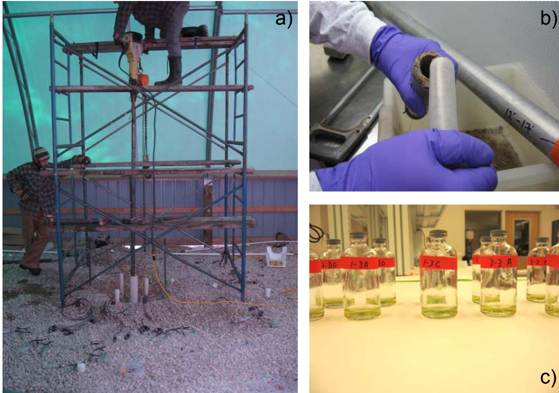
Figure 1.4: Core extraction for biomass analysis was done by hammering aluminum core sleeves into the subsurface (a). In the lab, the cores were sectioned at ~ 25 cm intervals and the centers were removed with a modified syringe barrel leaving behind a small rind in the core sleeve (b). Core centers were freeze dried and homogenized for later phospholipid extraction and spectrophotometric quantification to estimate the total viable biomass per gram dry weight sediment (c).
