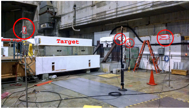
FIG. 1. The T576 experimental setup. The large white rectangular polyhedron at the center is the HDPE target. The beam enters from the left, with the entry point shielded by aluminum sheeting in an effort to mitigate transition radiation (TR). The circles (red) indicate the receiver/transmitter antennas. Second from left is the transmitter; the others are receivers.
