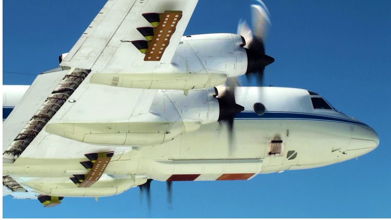
Figure 3.1: Installed RDS subarrays on the P-3 aircraft. Image courtesy of Rick Hale, 2011.
